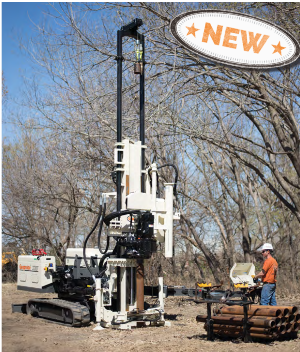
Kyle Riedel, Lead Engineer for the DT60 system, works at the controls of a 3230DT while 6.0 in. casing is driven in the early stages of sample collection. DT60 tooling was designed specifically to withstand the additional percussion force of the 3230DT and 8040DT rigs.
