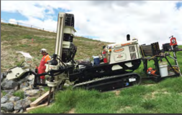
CPT testing for compaction. PRO-DRILL collects geotechnical data to confirm that the build/design of a fill site met requirements set for the site and could be signed off as completed to specifications. The site was a gully on a steep slope that was cut to bedrock, and was filled and compacted with the spoil of a large, new service trench upgrade close-by. Completing this testing eliminated the need to move a large amount of soil offsite for disposal. "The small footprint and stable platform of the 6622DPT rig gave us confidence to access the steep sloping site to complete the testing," reports Kris Hines, PRO-DRILL Driller/CPT Operator. "Bigger machines would slip and slide at this site and not be able to set up level to push the probe successfully."
