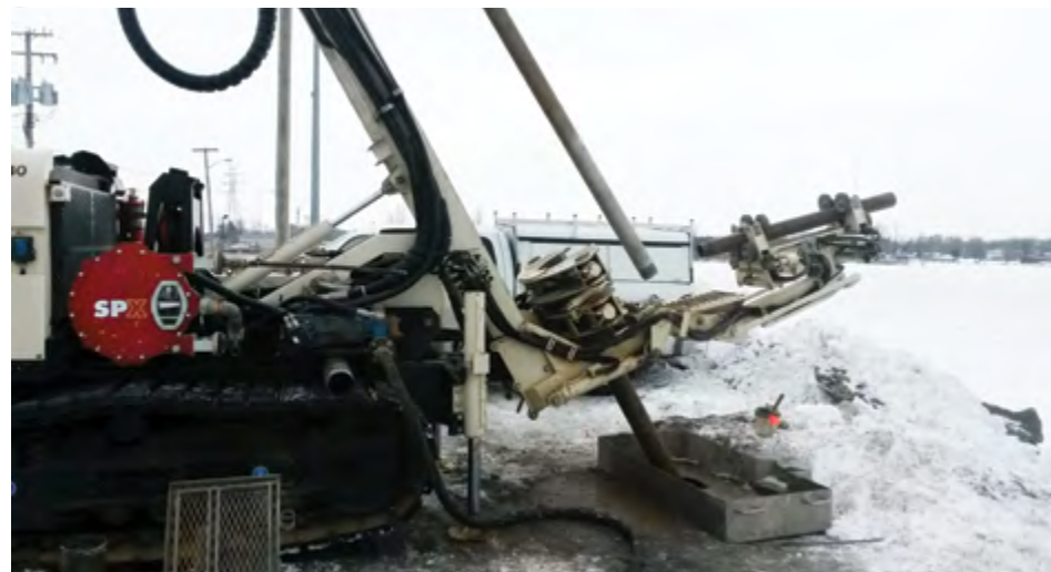
The Stearns Field Team has the 8140LS set up to take a second sample that would be chased by 6-in. rods.
