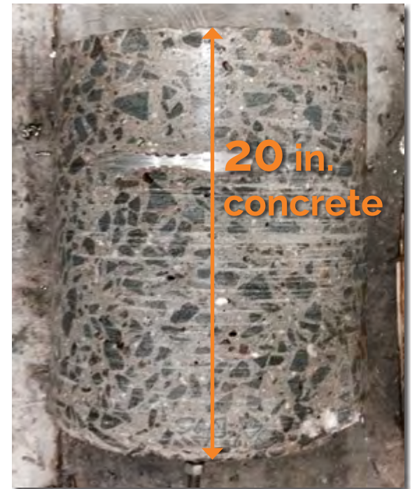
First Job. The AEAC Field Team took advantage of the adjustability of the hose pump and water swivel on the 3230DT to core through 20-in. thick concrete (above) flooring inside an aerospace metal recycling facility (left).
