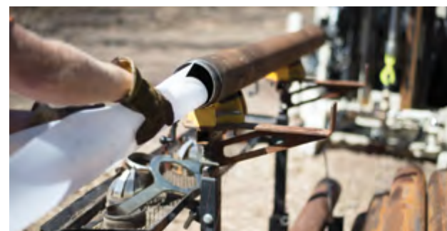
A new and innovative optional liner system for the DT60 decreases operating and shipping costs. Conventional liners are shipped in extremely large boxes. One hundred feet of DT60 liners comes in a box not much larger than a small microwave. Plus the liners can be re-used (when permitted), and they are easily recycled.
