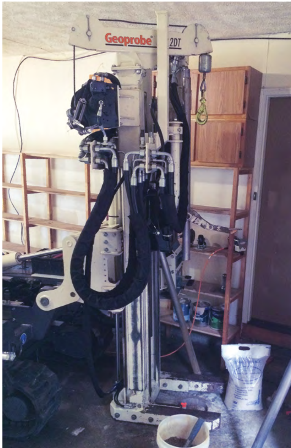
Enviro-Dynamics takes their 6712DT inside an 8-ft. high garage after a low-clearance cylinder was added to install a 1-in. diameter permanent monitoring well. Their working clearance was less than 2 inches, but the project was completed without damaging the ceiling of the garage.
