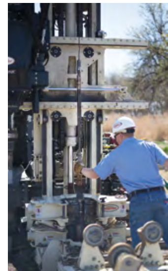
(right) A wireline overshot is released from the modular weight assembly during the sample collection process. The use of the winchline for retrieving sample sheaths reduces 'trip in' and 'trip out' times significantly.
