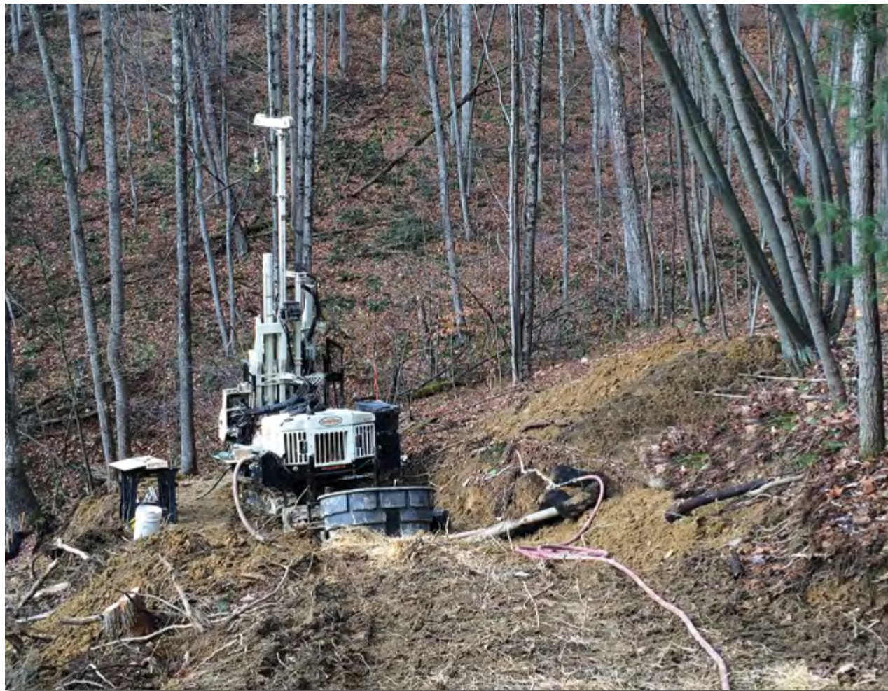
EnviroProbe’s 7822DT cored borings of 46 ft., 50 ft., 85 ft., 114 ft., 127 ft., and 190 ft. in the Monongahela National Forest.
