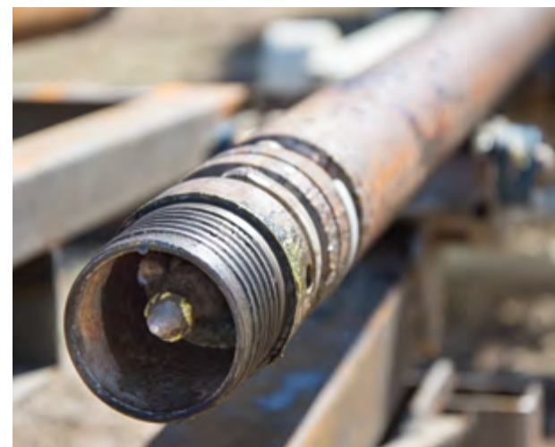
(above) The modular weight assembly, with the overshot 'spear' visible inside the weight drive head, prior to being lowered downhole. The modular weight assembly consists of two, 150-lb. weight segments coupled together and a threaded head and overshot spear.
