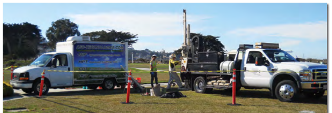
Environmental Control Associates utilized a Geoprobe® 6600 to push the MiHpt probe at 15 of the MiHpt locations. ECA used the Geoprobe® DT22 Soil Sampling System to collect soil cores to confirm the MIP responses and verify what the HPT pressure responses and EC logs were revealing about the local formation.
