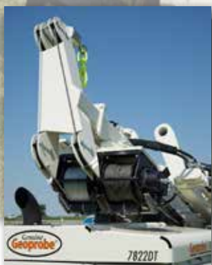
The new dual winch kit for the 7822DT consists of one winch containing 75 feet of 5/16-in. wire rope, and a second winch containing 250 feet of 3/16-in. wire rope.
