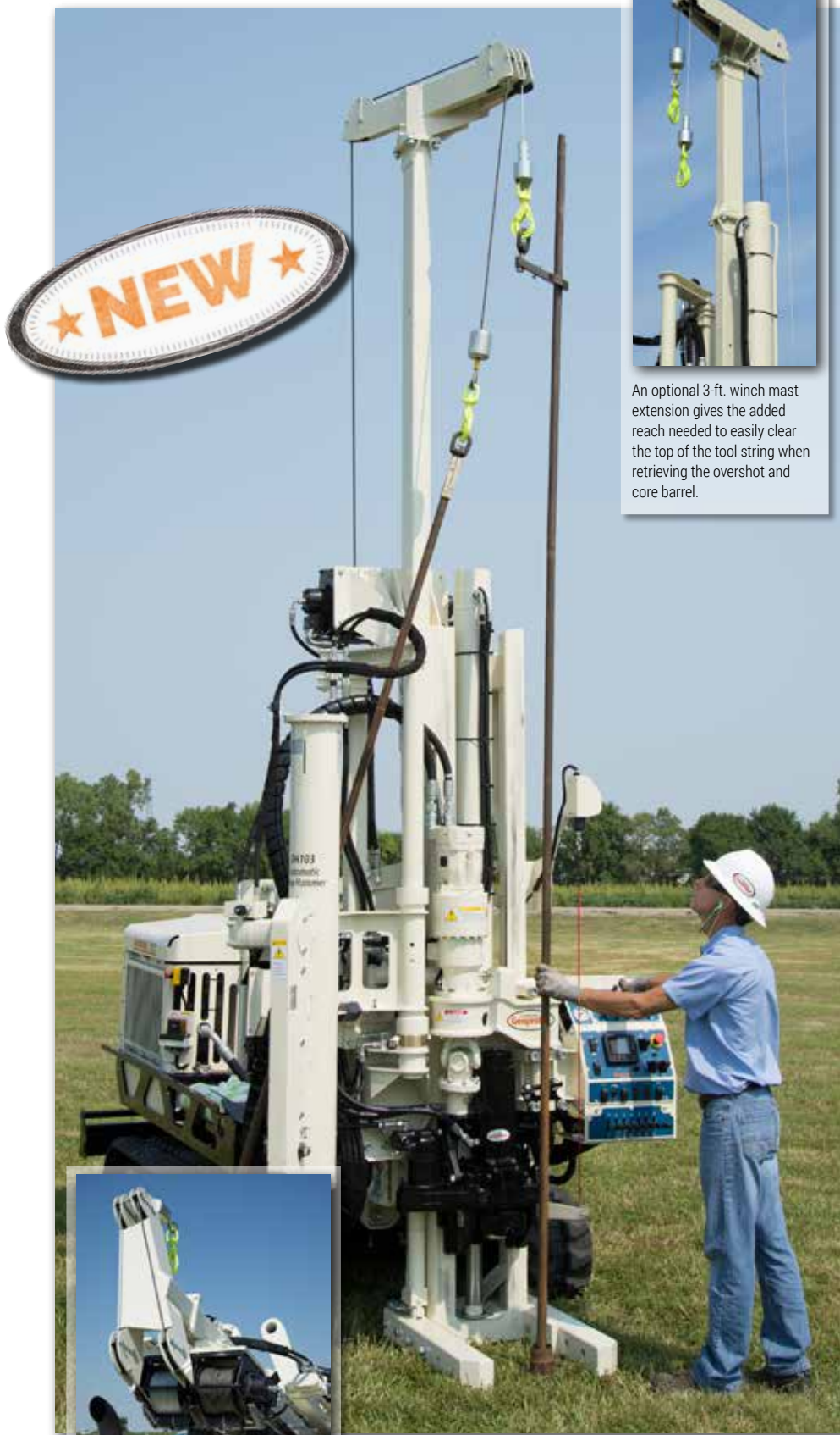
The new dual winch kit for the 7822DT consists of one winch containing 75 feet of 5/16-in. wire rope, and a second winch containing 250 feet of 3/16-in. wire rope.
