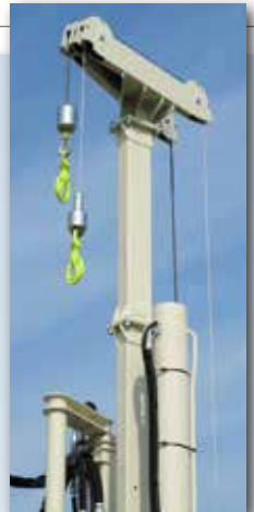
An optional 3-ft. winch mast extension gives the added reach needed to easily clear the top of the tool string when retrieving the overshot and core barrel.
