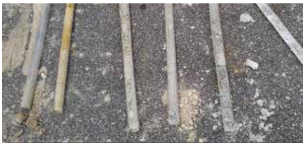
Using the robust MC5 sampler and 2.5-in. rods, the 3230DT was able to easily get through the dense clays and weathered limestone.
