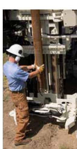
Pushing 6-in. casing is a breeze with the 3230DT. You'll find DT60 to be one of your most-used tooling systems because it's so easy to use.
