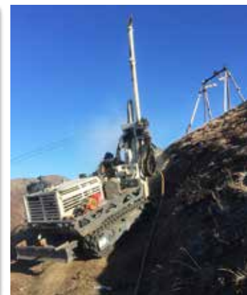
Darrin VanDehey advances air rotary tooling with the 6712DT sitting at a substantial angle.
