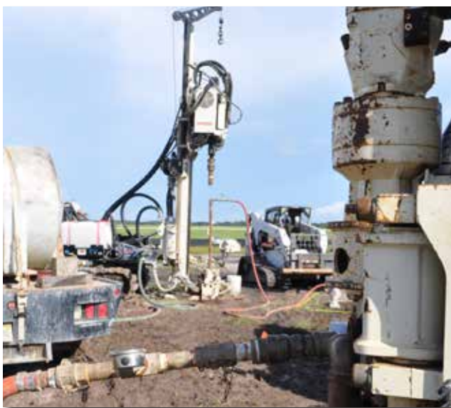
(above) A 7822DT drives injection tooling in the overburden soils.
