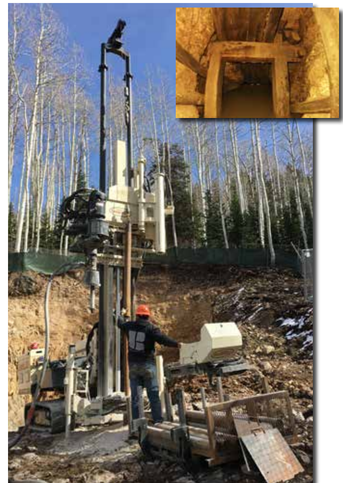
Nate Salazar uses the 3230DT to locate an abandoned mine tunnel below a proposed new hotel project in the Wasatch mountain range east of Salt Lake City. The inset above shows one of the images taken downhole of the tunnel.
