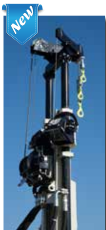
NEW! Triple Winch Option. One big winch for pulling, an intermediate winch for pulling and lifting tools, and one for wireline work.
