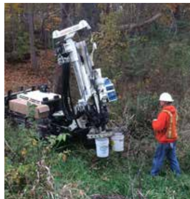
Steve Baltus navigates the 6712DT through some rugged terrain to complete discrete groundwater sampling up to 90 feet using an SP16 sampler.
