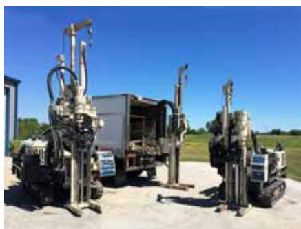
The Enviro-Dynamics Geoprobe® fleet: 7822DT, 6600 with PC111 carrier, and 6712DT with low clearance option.
