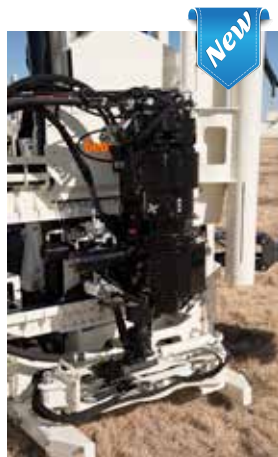
NEW! 6-Speed Combo Head Option. Increased torque (8,700 ft-lbf maximum torque) for augering. Increased speed for rock coring (900 rpm maximum rotation)..
