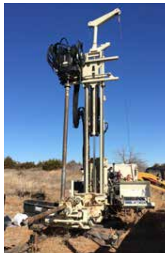
An 8150LS, owned by Associated Environmental Industries in Norman, OK, runs SDT60 and a 6.0-in. Weighted Wireline system.
