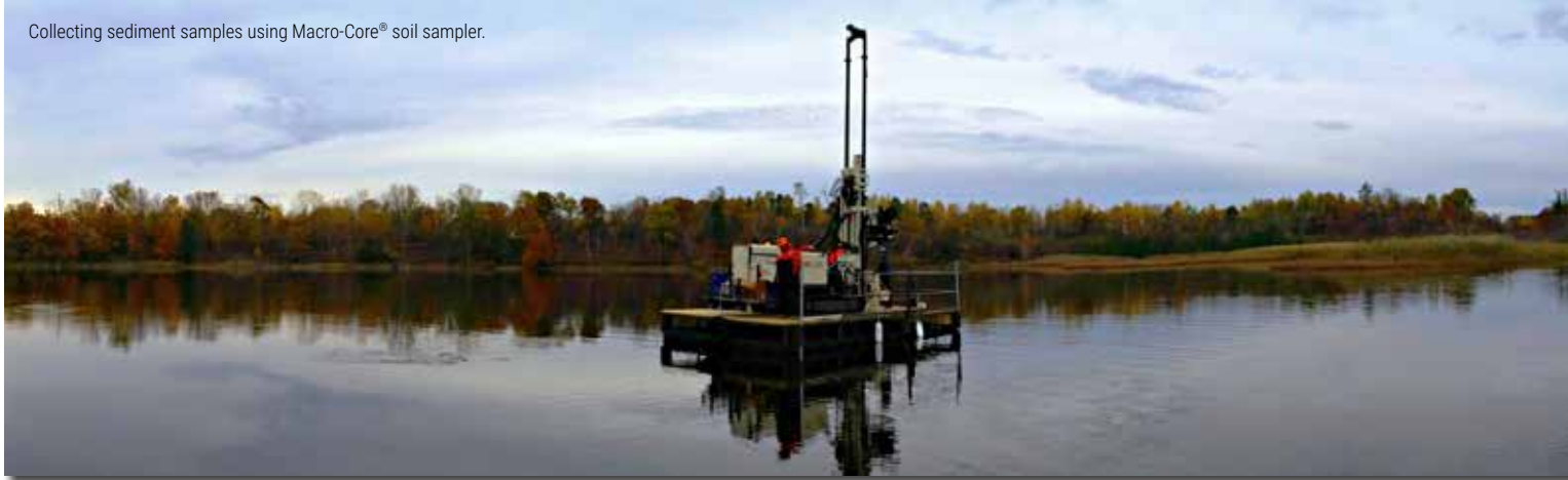
Derek Fennell and Bob Gannon complete split spoon, Macro-Core® soil sampling, and wireline rock coring on an earthen dam.
