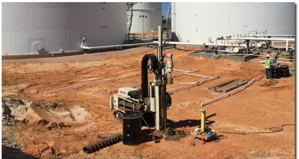
Sampling and site delineation after an ethyl alcohol leak near the Gulf Coast.
