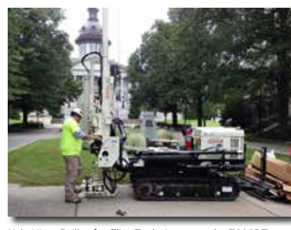
Kyle King, Driller for Elite Techniques, and a 7822DT are soil sampling on the South Carolina State House lawn.
