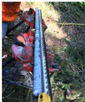
A 5-ft. rock core collected by DJ Wardwell, Operations Manager, with a 6712DT.
