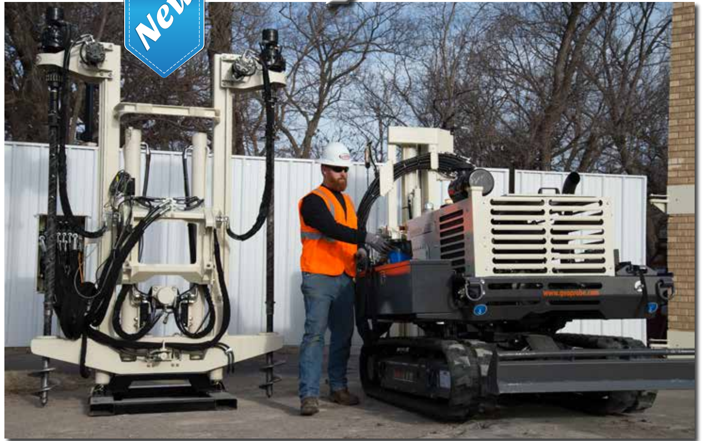
Josh Dreiling, Geoprobe® Engineer, prepares to move the 6712 power unit module away from the direct push mast and connect it to the 20-ton CPT Press unit (left). The 20CPT Press has 20 tons of hydraulic downforce, and features two built-in soil anchors, adjustable feed rate, and top and bottom hydraulic rod clamps.
