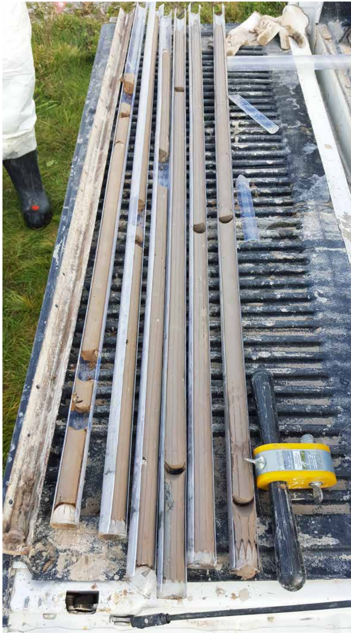
Filled DT22 soil core liners recovered by GeoServ using Geoprobe® liners and a 6620DT. The integrated core catchers in the liners (shown at end of each liner) keeps the sample from falling out the bottom of the liner as the core is retracted.
