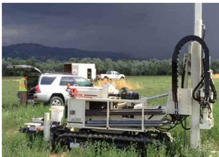
West Bountiful, UT. A 6620DT, EarthProbe's most used piece of equipment because of its versatility, completes a soil and groundwater investigation.
