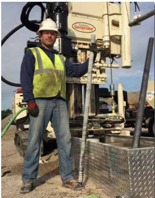
John Durbin says it’s a mighty fine 5-ft. rock core pulled with their 3230DT! John and Josh Caldwell spent a couple days in Kansas training on their new sonic, and successfully pulled this sample at their first rock coring site.
