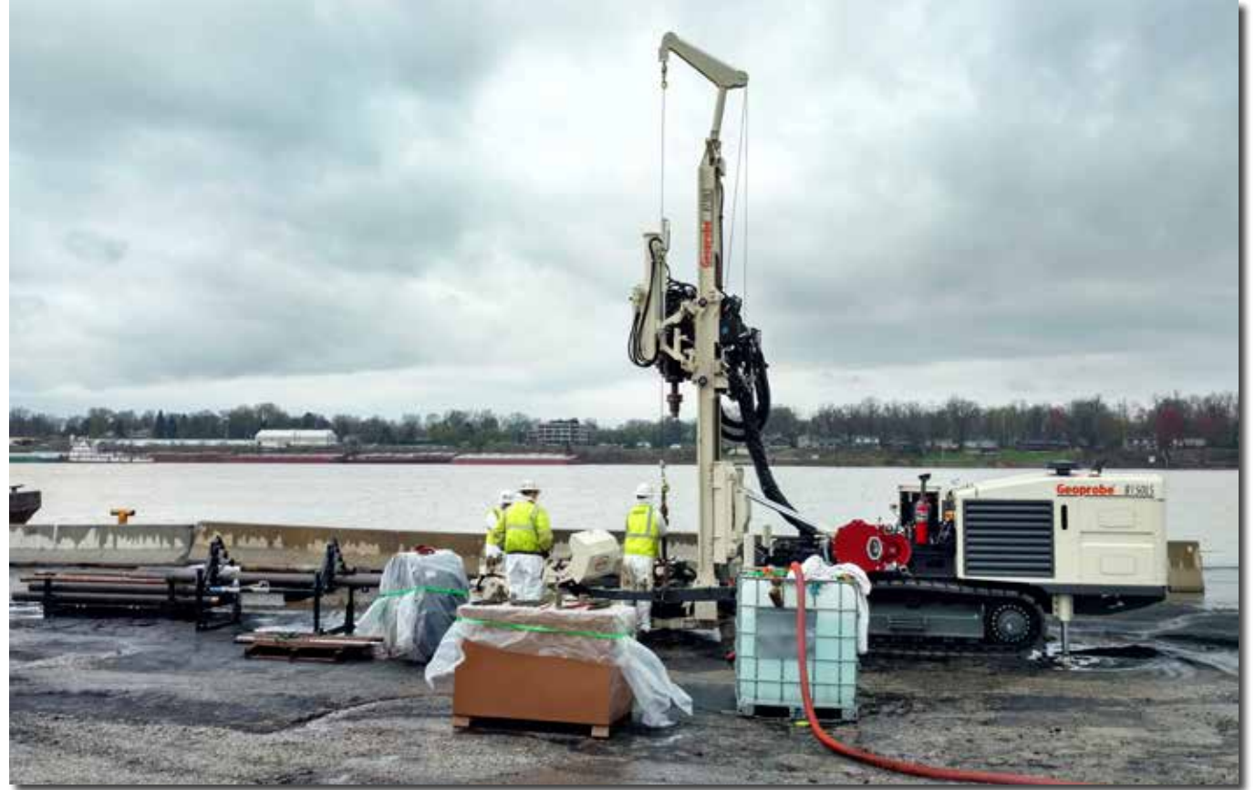
EnviroProbe Integrated Solutions, Inc., in Nitro, WV, initiates their new Geoprobe® 8150LS Rotary Sonic at a contaminated site requiring geotechnical work near Louisville, KY.
