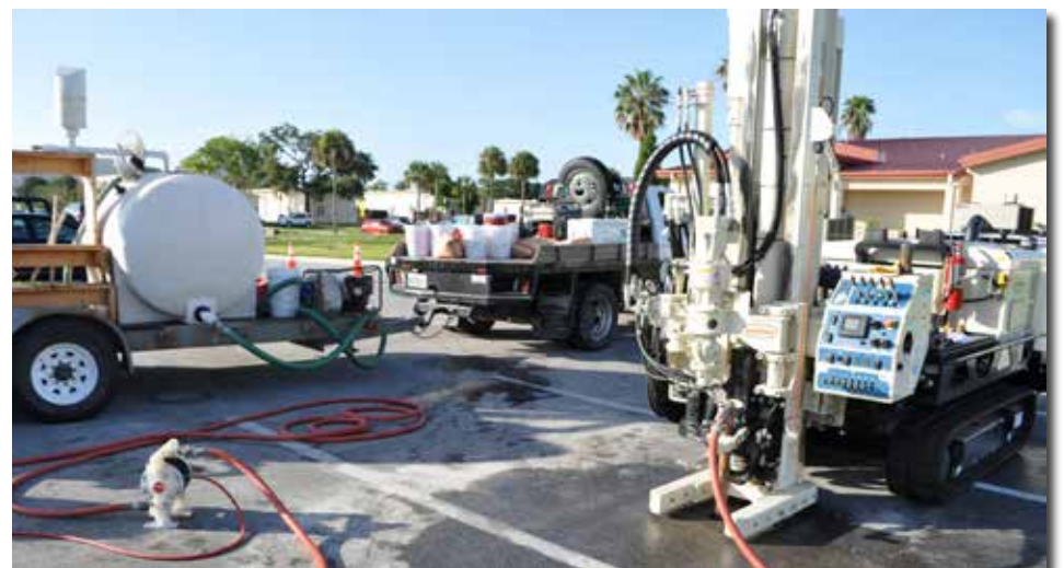
(above) A 7822DT drives injection tooling in the overburden soils.
