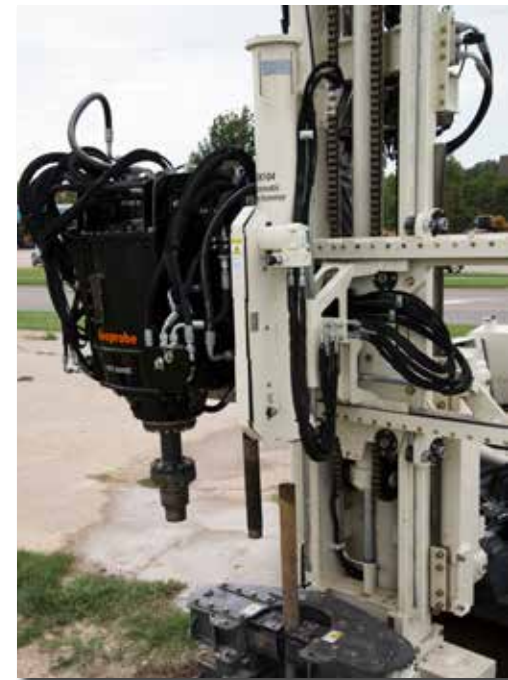
The Automatic Drop Hammer option for the 8150LS sonic allows for collecting split spoon samples and other geotechnical applications.
