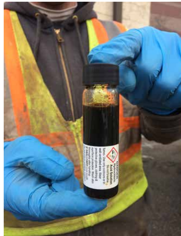
Confirmation sampling conducted by S2C2 using an SP16 groundwater sampler at Location 17 confirmed the presence of DNAPL.
