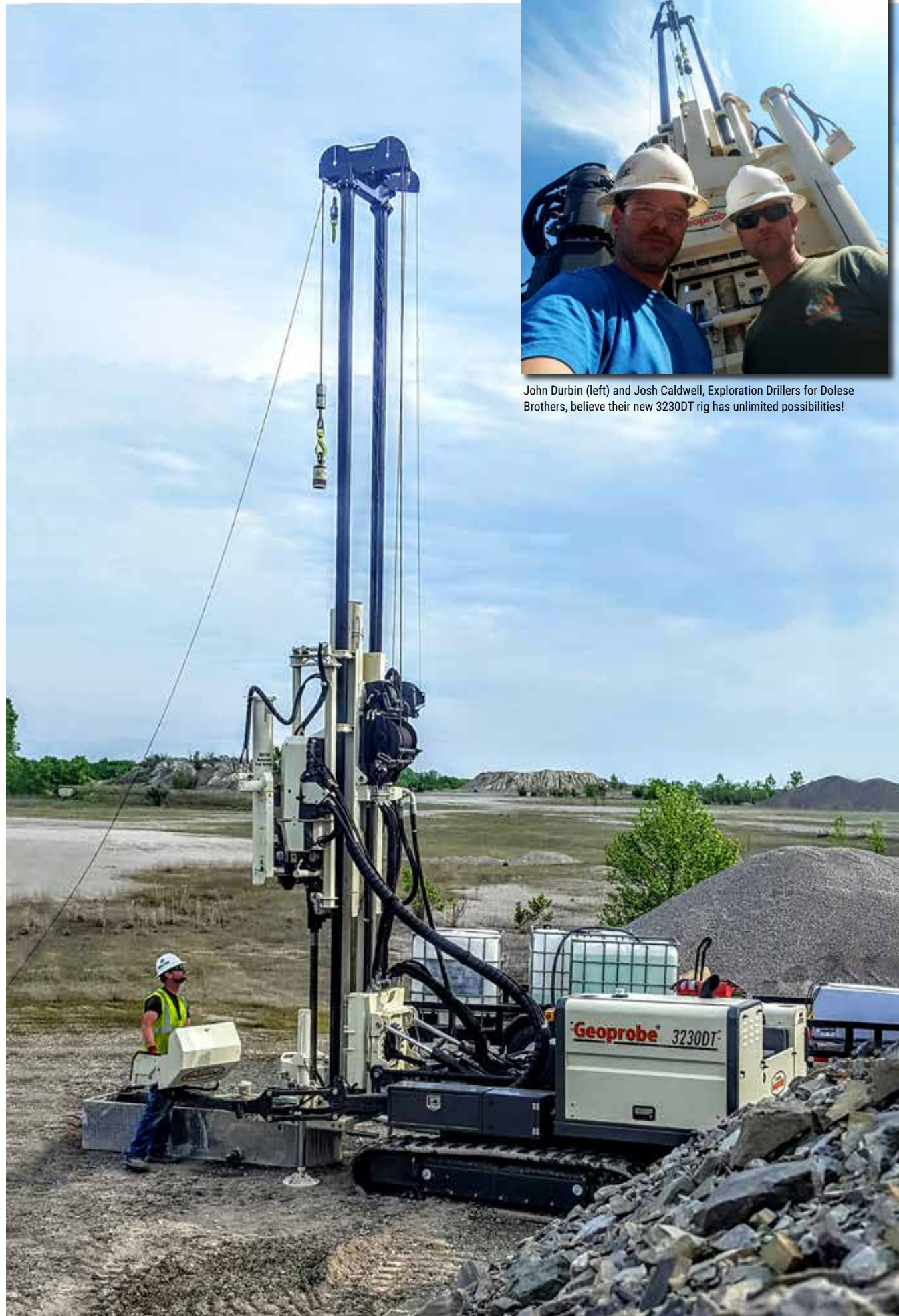
Josh Caldwell, Dolese Brothers, is at the controls of the 3230DT in southeastern Oklahoma. DT35 sample cores will make for easier sampling and provide the company with high-quality information to know what’s in their quarries and to know where to blast.
