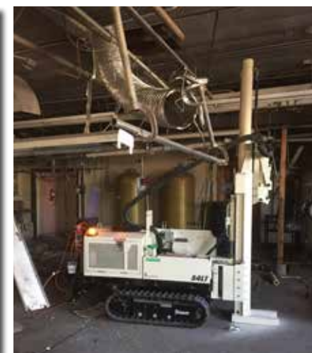
Salt Lake City, UT. A 54LT excelled inside a former dry cleaners facility for a soil and groundwater investigation.
