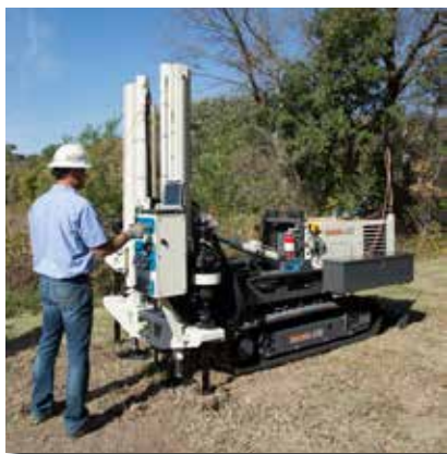
Doug Koehler, Geoprobe® Sales, operates the 20CPT Press on the 67 Series power unit. This 20-ton CPT Press is another way for you to economically diversify your business with Geoprobe® products.
