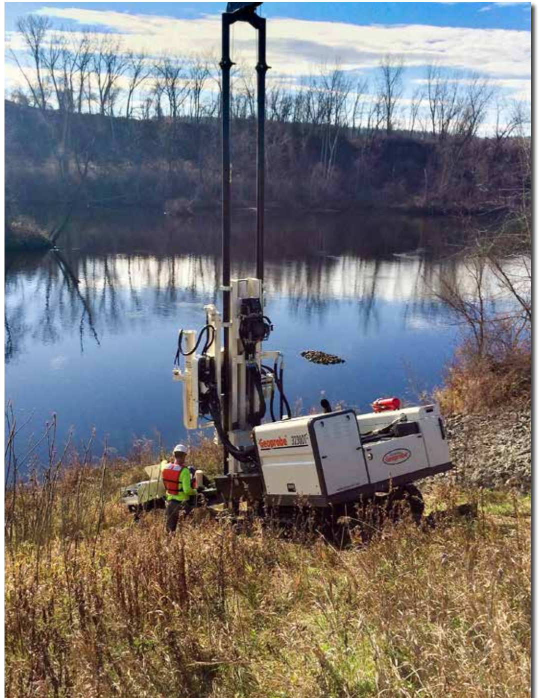
Derek Fennell and Bob Gannon, Drillers with Aztech Environmental Technologies, use the 3230DT for split spoon, Macro-Core® soil sampling, and wireline rock coring on an earthen dam.
