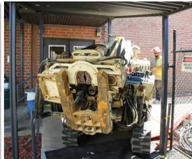
(above and below) Drew Small with TRS contacted Geo Lab to assist with ERH electrode installation at an active manufacturing facility near Murphy, NC. For this most recent phase, Geo Lab installed supplemental electrodes, as well as obtained continuous soil samples with soil temperatures around 200 degrees F. A 7822DT pulled the continuous hot soil samples, from 100 ft. bgs, by advancing a Macro-Core® sampler with stainless steel liners to withstand the heat. Following the sampling, Geo Lab installed multiple electrodes to greater than 100 ft. using hollow stem augers, requiring very careful handling of the steaming mud. After completion, Drew Small said that in the early stages of the project he had his doubts as to whether the scope of work could be completed. "I was impressed with the capability of the rig and your guys during this install," he said. "I wasn't sure it was possible."
