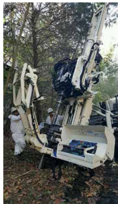
Because of the rig's tracks, M&W's 8150LS can access difficult terrain.
