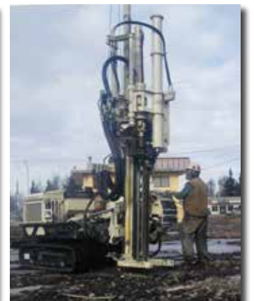
Richard Banzhaf, Driller, collects 3-in. MC7 soil samples using the 7822DT.
