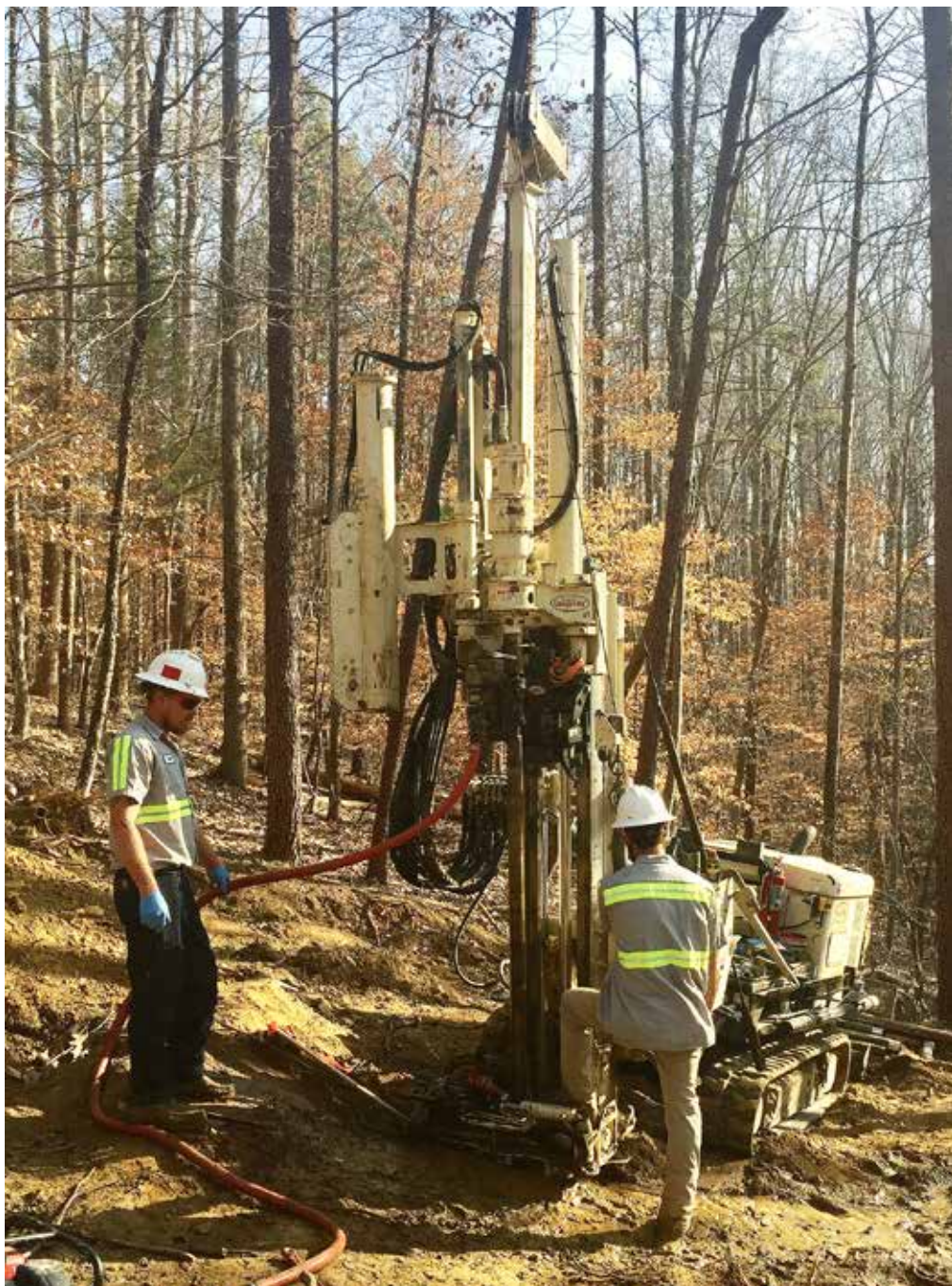
Tyler Felder and Randy Eddings use the 7822DT to rock core deep in the woods near Reidsville, NC
