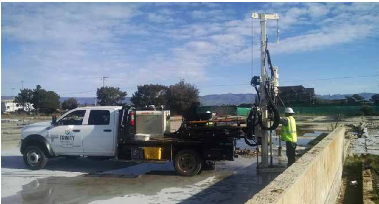
(above) Eric Choi, at the controls of the Trinity Drilling 7800, using concrete coring to retrieve soil samples at a Watsonville, CA, commercial development. (below) Eric Choi and Drew Gagnier complete a soil and groundwater investigation at a residential site in East Palo Alto, CA.
