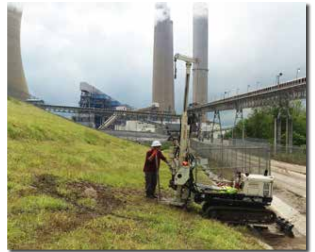
Ron Dutmer, Driller's Helper, and Tom Ulrich, Driller/Crewchief with Stearns Drilling use a Macro-Core® sampler in Ohio to retrieve bio samples from screened intervals of a nearby well. Each sample had to be capped and sealed as it was removed from the core liner.
