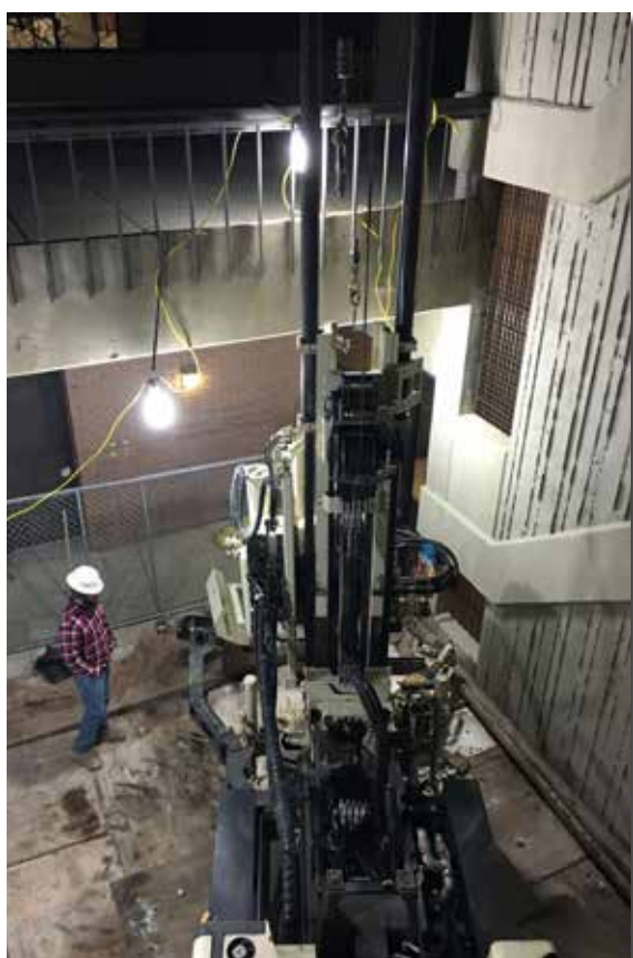
Thomas Maughan surveys the AGEC 3230DT and his work area during a site investigation surrounding an office tower in Salt Lake City.
