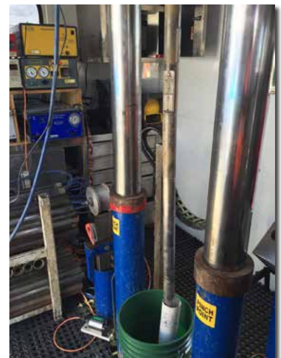
MIP and CPT tooling ready for deployment.
