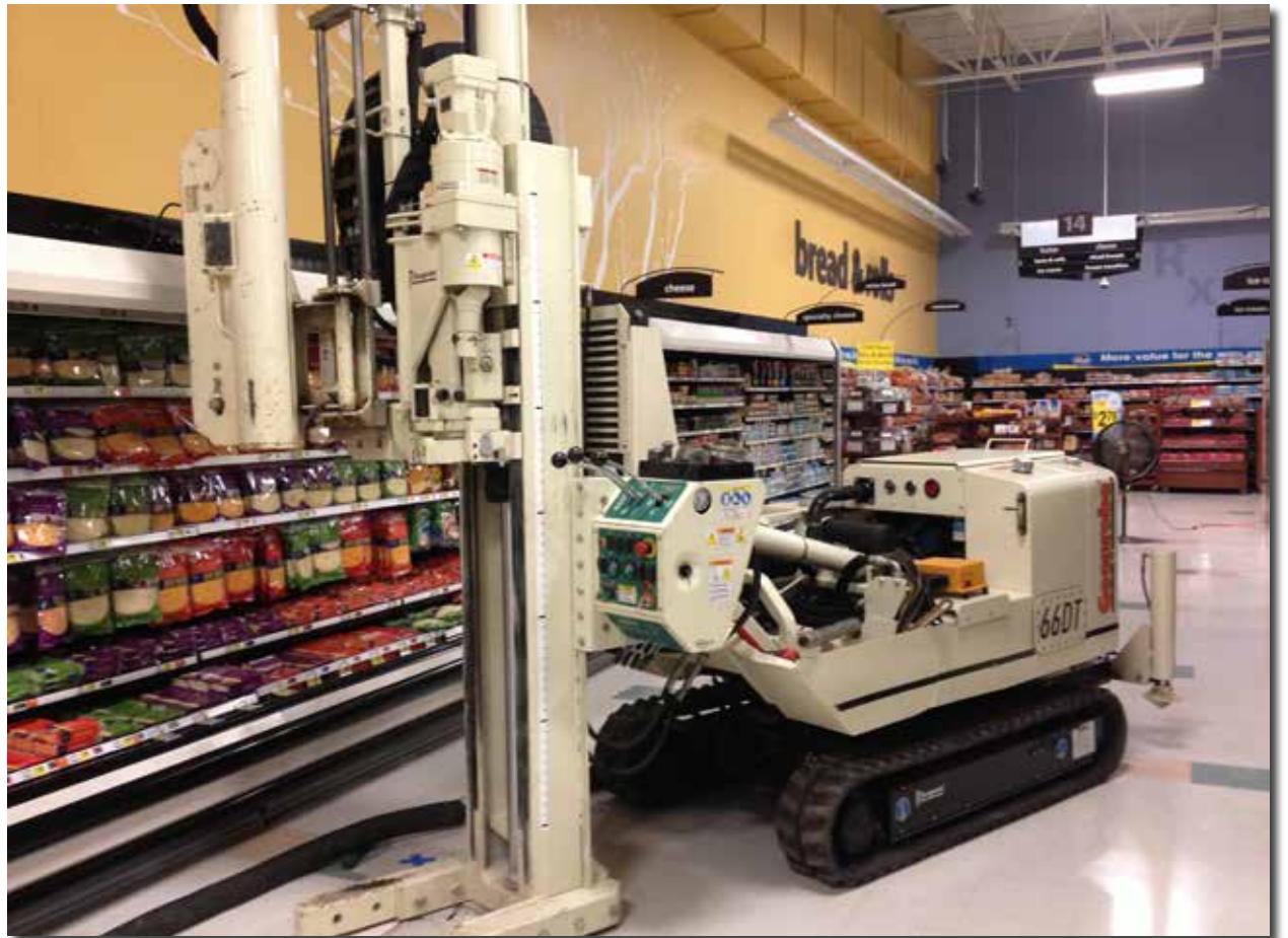
Nearly as shiny and clean as it was coming out of the factory, Geo Logic's 66DT retrieves soil samples inside a grocery store (after hours).
