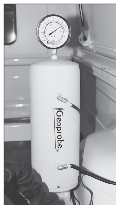
Vacuum/Volume System tank and gauge.
