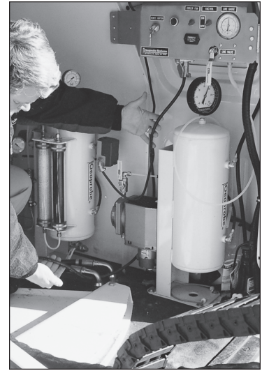
Vacuum/Volume System mounted in a Geoprobe-equipped standard cargo van.
