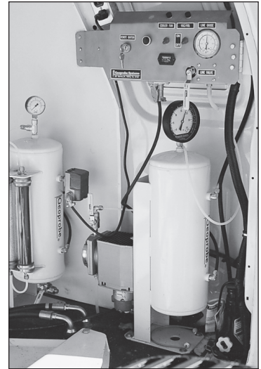
Mountable Vacuum/Volume System was designed for extraction of soil gas samples from probe cavities.
