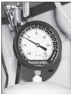
Vacuum gauge calibrated in kPa and volume in liters.
