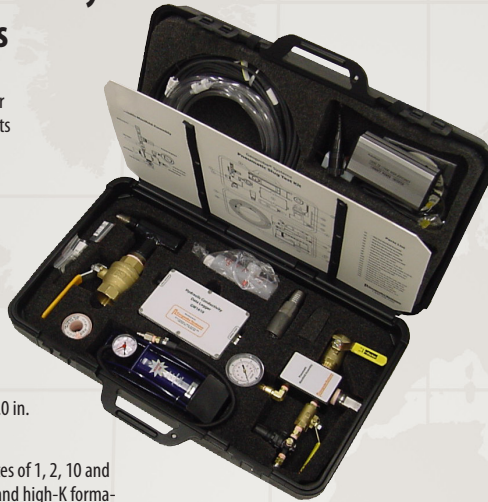
Hand pump has a valve that allows for changing from pressure to vacuum so that rising or falling head tests may be performed.
