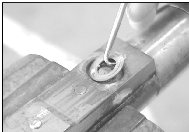
Figure 6.2 Remove and discard the copper washer.
