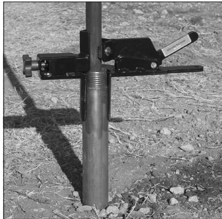
Figure 1: Adjustable rod holder installed on a 2.25-inch outer casing.
