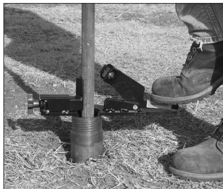
Figure 3: Lightly step on the holder handle to open the rod holder jaws.
