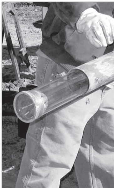
Figure 4.9. Liner, core catcher, and liner retainer are slid into sample sheath.
