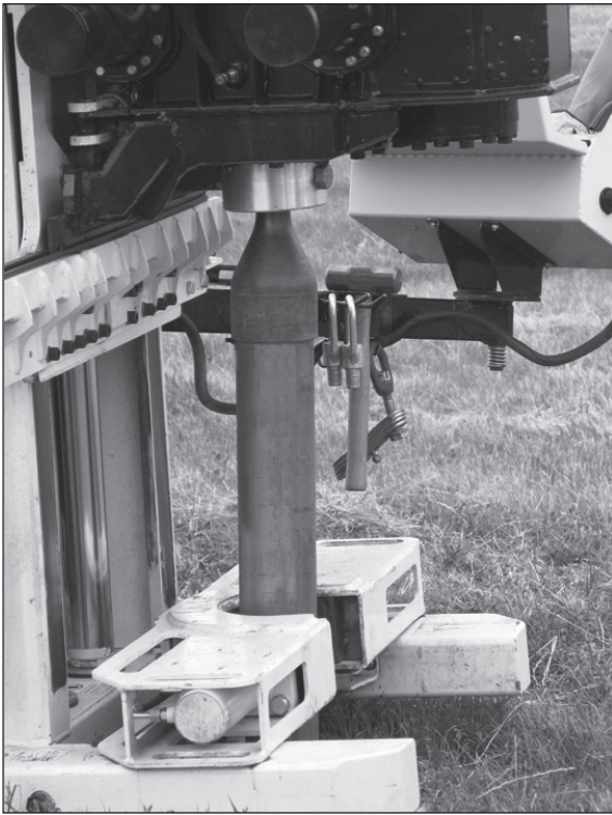
Figure 4.15. Advancing the DT45 Sampler
