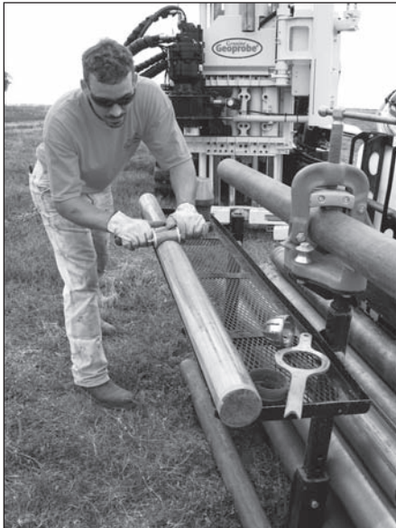
Figure 4.22. Use the DT45 Liner Cutter to safely expose the sample.
