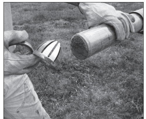
Figure 4.21. Remove liner retainer and core catcher.
