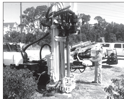
Figure 4.14. DT45 Sampler is centered before initial push.
