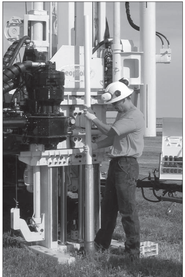
Figure 4.24. A Geoprobe® 2.0-in. Prepacked Screen Monitoring Well can be installed using the DT45 Soil Sampler.
