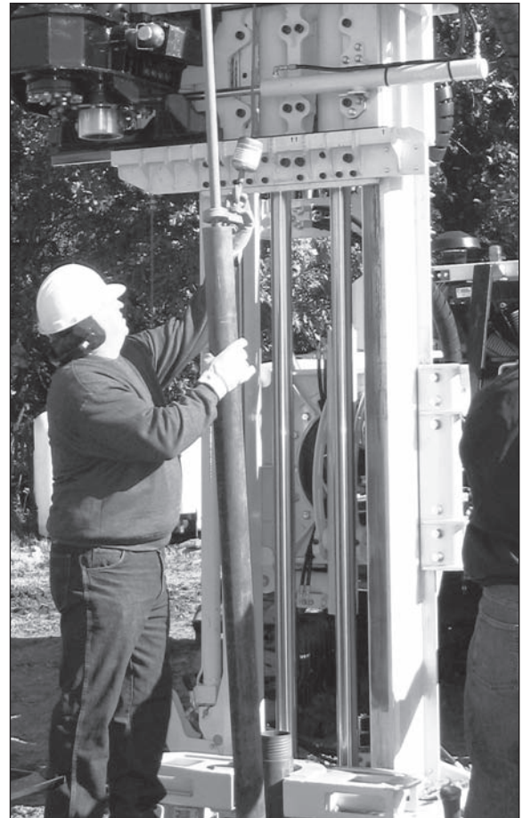
Figure 4.18. Inner rods and sample sheath are retrieved.
