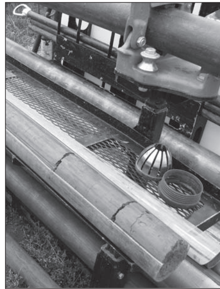
Figure 4.23. Slit liner exposing the sample.
