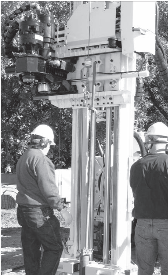
Figure 4.17. The adjustable rod clamp and leaf puller can be used when retrieving the sample.
