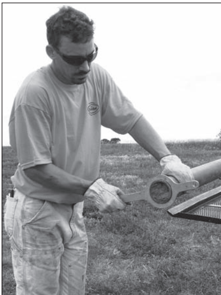
Figure 4.19. Remove the liner retainer with liner retainer wrench.
