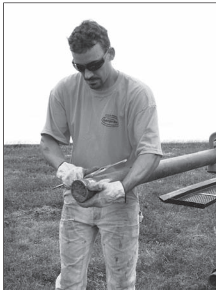
Figure 4.20. The wrench can be used to gently knock off the retainer.
