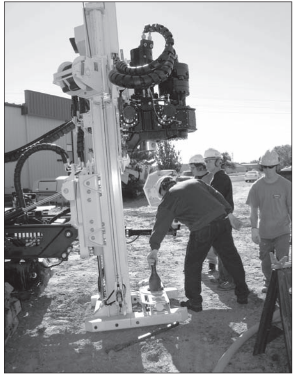
Figure 4.16. Remove drive cap to provide access to inner tool string.
