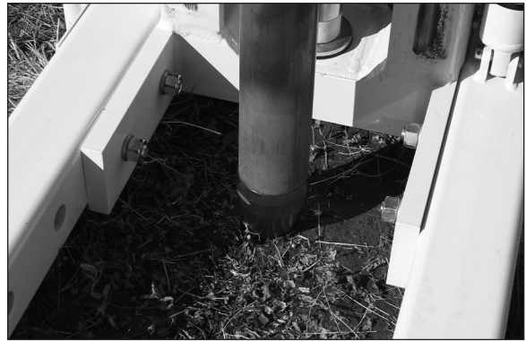
Figure 4.14. The probe rod should be centered between the toes of the probe foot.
