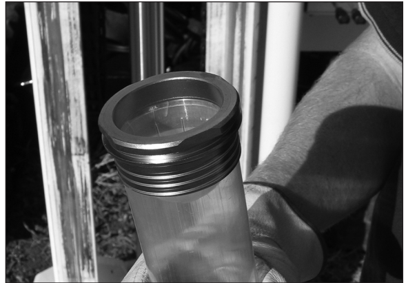
Figure 4.7. The retainer ring is placed on the end of the liner.
