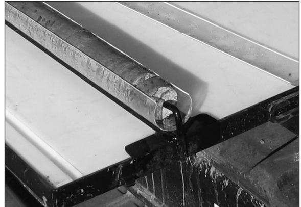
Figure 4.20. The core is exposed by the DT325 Liner Cutter.
