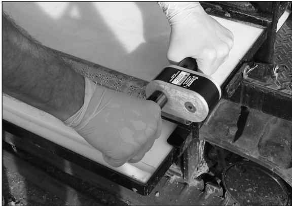
Figure 4.19. The DT325 Liner Cutter is used to safely make a longitudinal cut on the sample.
