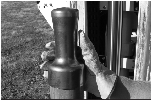
Figure 4.13. Place the threadless drive cap on the 3.25-inch probe rod.
