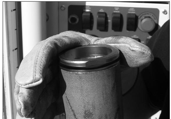
Figure 4.9. Tighten the retainer ring by hand.
