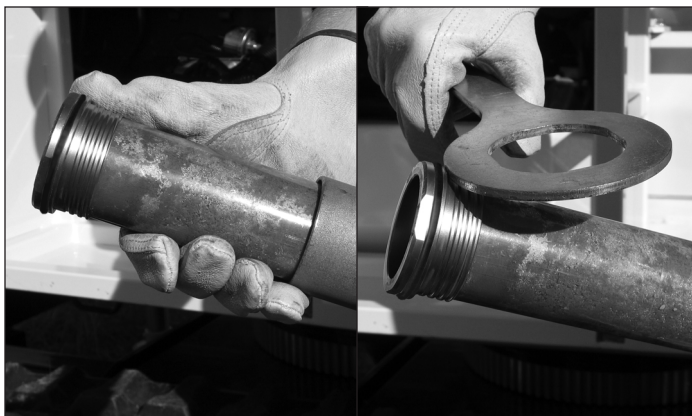
Figure 4.17. The retainer is removed from the sheath, either by hand or with the retainer wrench. Gently tap the retainer with the wrench to remove it from the liner.
