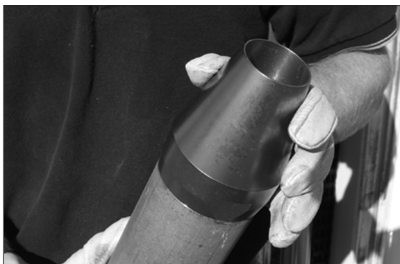
Figure 4.11. The cutting shoe is threaded onto the 3.25-inch probe rod.
