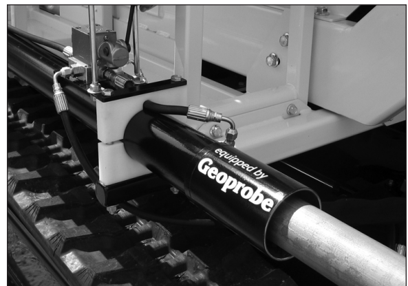
Figure 4.18. The Hydraulic Liner Extruder helps remove the liner.
