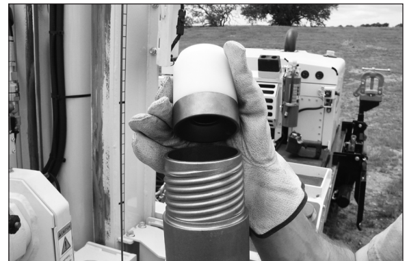
Figure 4.12. A DT325 Buffering Centering Drive Cap (37708) is placed on the DT325 Drive Head.
