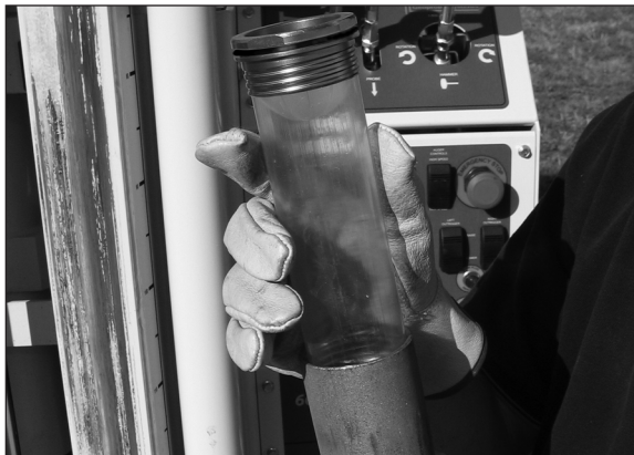
Figure 4.8. The liner and spacer ring are slid into the sample sheath.
