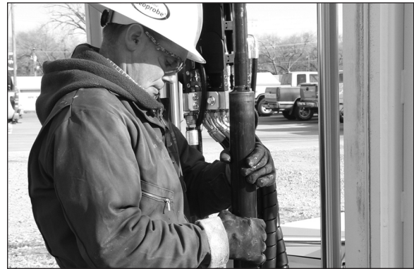
Figure 4.16. The 1.25-inch light-weight center rods are pulled along with the sample tube.
