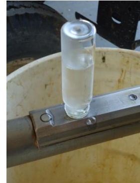
Figure 5.5: 40ml vial of working standard inverted onto membrane
