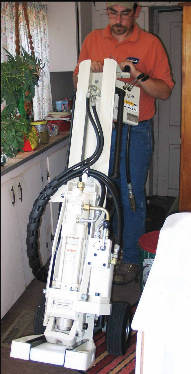
Collecting geotechnical samples for a new elevator shaft.
