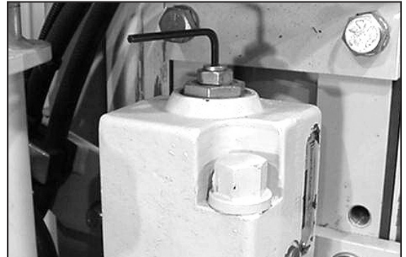
Figure 4: Remove cap from nitrogen charge valve.
