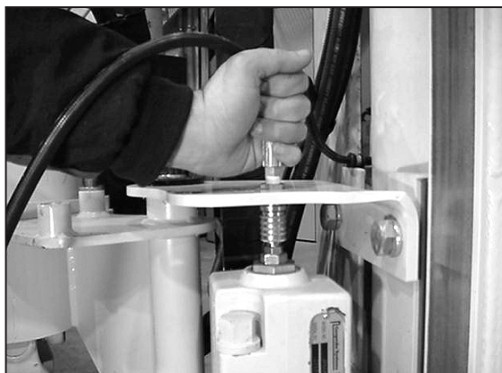
Figure 7: Push coupler onto quick connect nipple.
