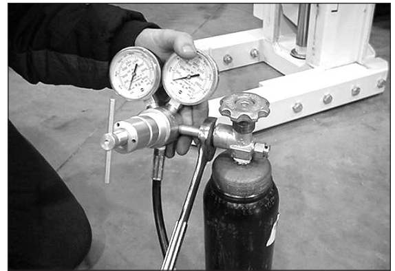
Figure 3: Attach regulator to cylinder.
