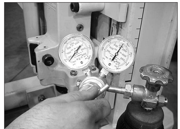
Figure 8: Adjust fill line pressure with the regulator.
