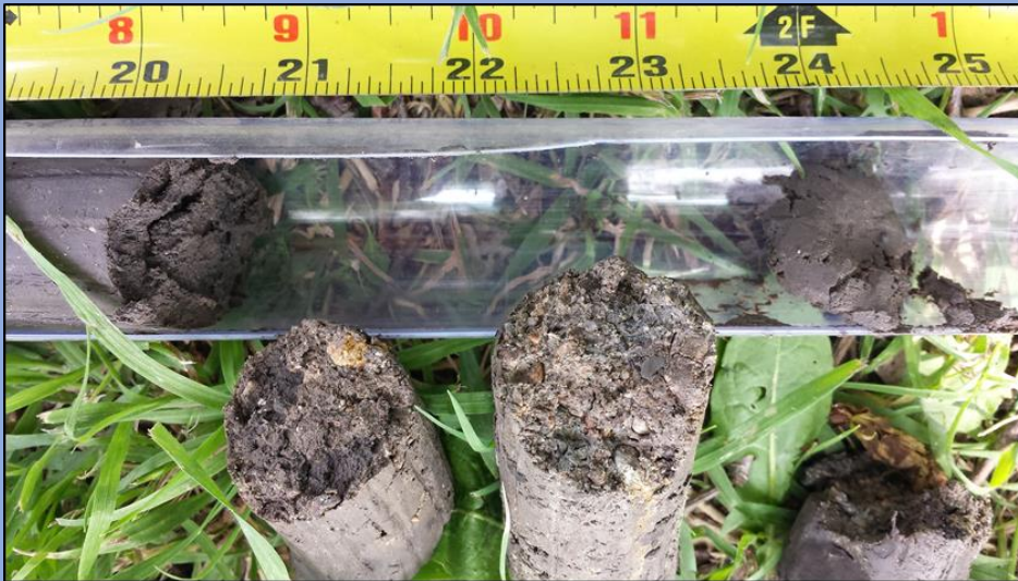
DT22 soil core from location exhibiting false positive response due to limestone clasts and caliche nodules.
