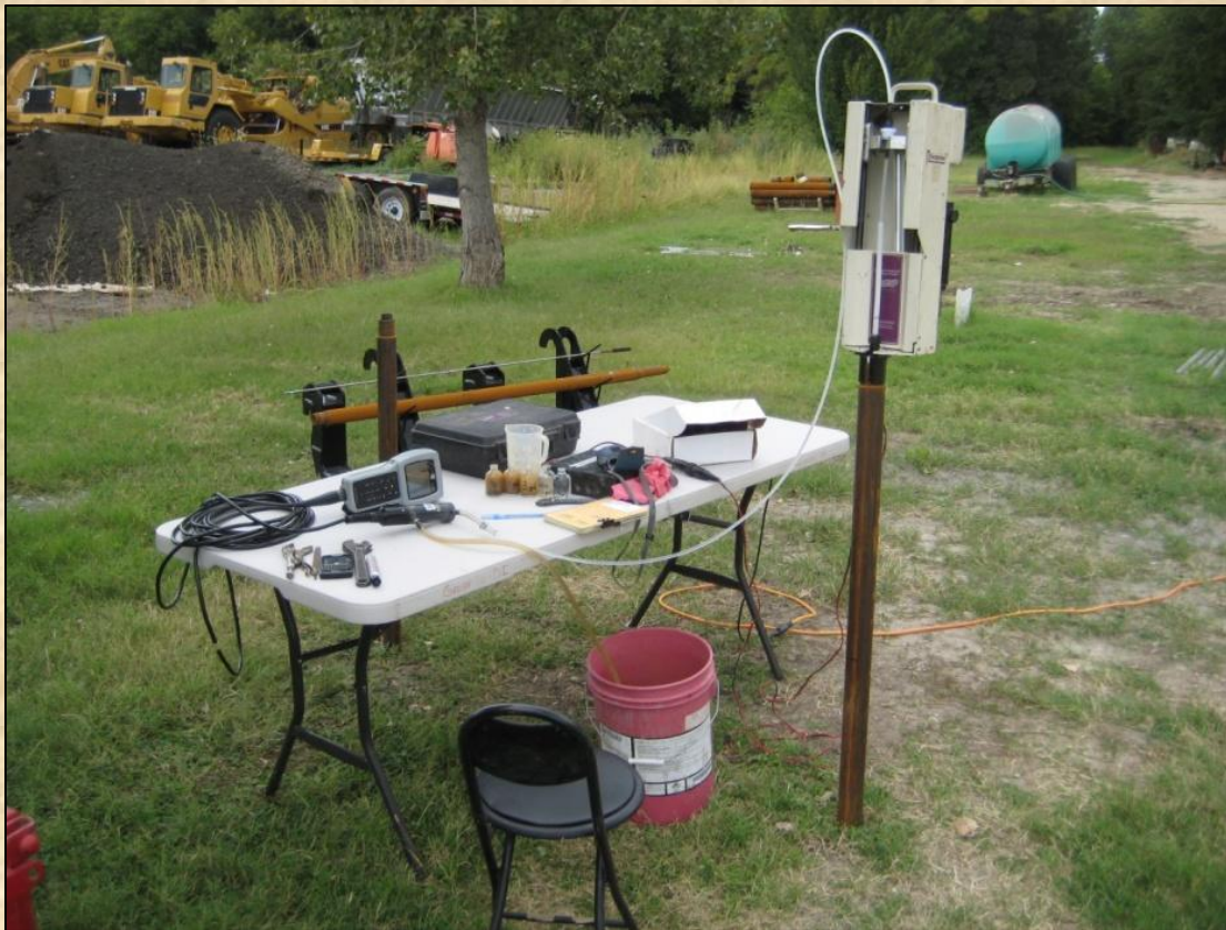
Monitoring water quality while purging
