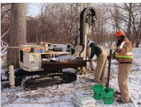
(below and lower right) Thiele Geotech uses their 6620DT to retrieve soil samples at the former Ash Lagoons near Omaha, NE. Redevelopment construction of the area will involve the excavation and disposal of approximately 8,200 cubic yards of soil. The field team members were Cory Bachman, Driller; James Beutler, Driller’s Assistant; and Dennis Anderson, Senior Geologist.
