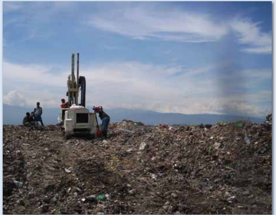
Omar Velazquez, EnviroTek's Geoprobe® rig operator, collects another soil core from the 500-acre Truitier Landfill near Port-au-Prince while a Haitian family watches. Over 90 acres of the landfill are currently used for the city's 1.3 million population and earthquake rubble.
