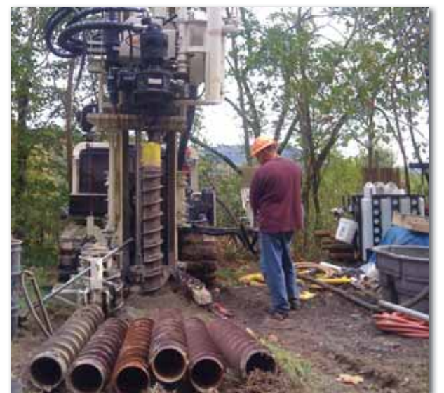
Dale Kestner Driller for EnviroProbe, augers to bedrock (approximately 40 ft) using the 8040DT.
