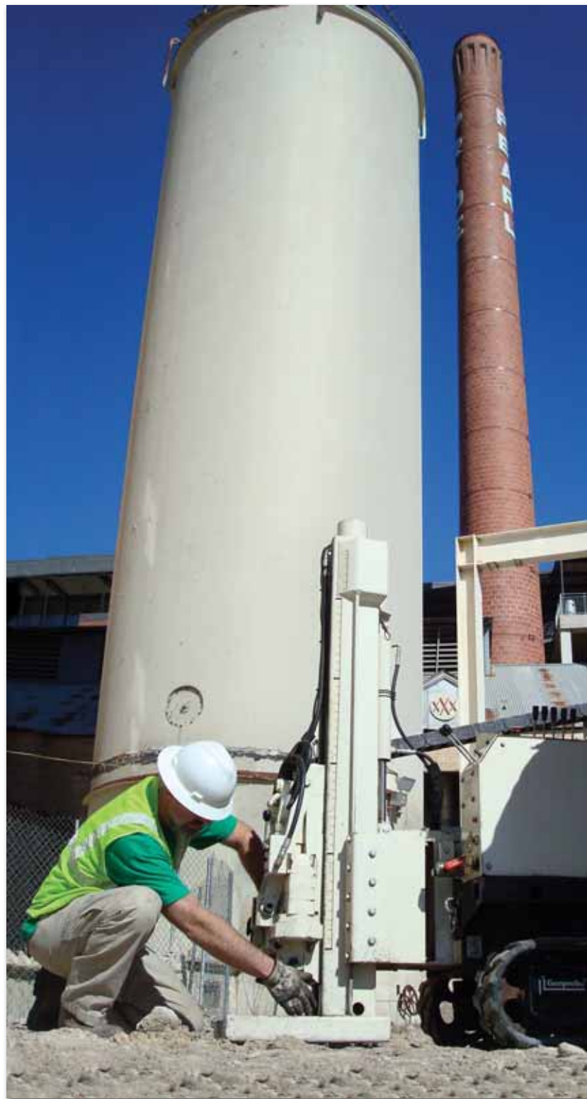
Because of its small size, the 54LT can easily maneuver within confined spaces ...inside and out...allowing the GeoTest field team to efficiently collect high-quality, limited access soil samples. (above) Alex Forhertz, GeoTest rig operator, uses the 54LT near the base of the former grain silo. The brewery's renovated smoke stack, constructed of curved clay tile, stands to the right. (right) At 34-inches wide, the 54LT fits easily through standard doorways. Ray Meinhardt (left) and Alex Forhertz, retrieve MCS soil samples through the concrete floor between the brewery's beer fermentation structures.
