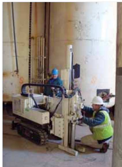
Because of its small size, the 54LT can easily maneuver within confined spaces ...inside and out...allowing the GeoTest field team to efficiently collect high-quality, limited access soil samples. (above) Alex Forhertz, GeoTest rig operator, uses the 54LT near the base of the former grain silo. The brewery's renovated smoke stack, constructed of curved clay tile, stands to the right. (right) At 34-inches wide, the 54LT fits easily through standard doorways. Ray Meinhardt (left) and Alex Forhertz, retrieve MCS soil samples through the concrete floor between the brewery's beer fermentation structures.
