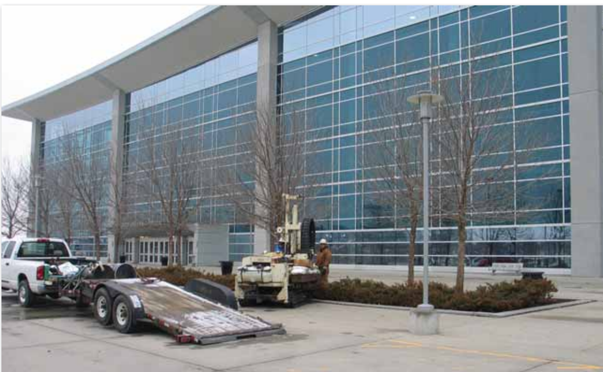
(top and above) Thiele Geotech retrieves SP16 groundwater samples as part of an ongoing monitoring program at the 1.1 million sq. ft. Qwest Center in Omaha, NE. The facility was built on a Brownfield’s site that was historically used as a railyard for the Union Pacific Railroad. Construction for the $290 million arena and convention center, which covers 100 city blocks, was completed in 2003. Cory Bachman, Driller, and Kyle Gappa, Driller’s Assistant, operate their Geoprobe® 6620DT. (right) Thiele Geotech’s field team and 6620DT completed geotechnical drilling services at the Creighton University Ryan Athletic Center in downtown Omaha. Six-inch augers were used to advance Shelby tubes to 20 ft.
