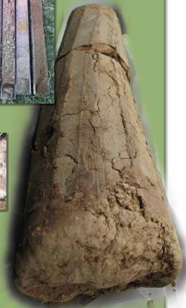
6-in. sonic core barrel sample collected using 8140LC Rotary Sonic.
