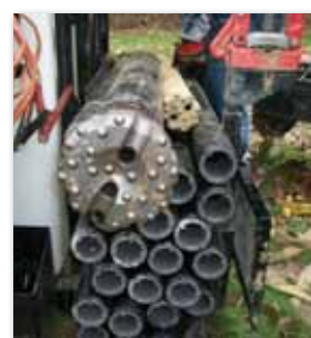
(left and below) EnviroProbe used a 6-in. downhole (DTH) hammer with an 8-in. bit and API IF rods to install the cased monitoring well. Dale Kestner, Driller for EnviroProbe, is at the controls of the 8040DT.
