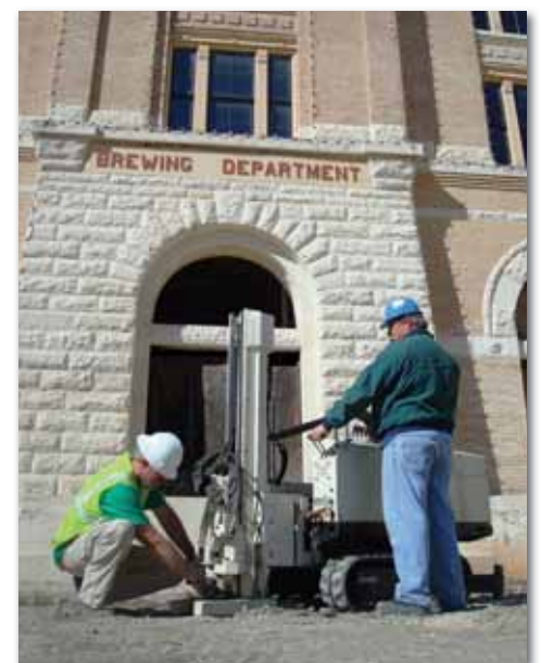
GeoTest used their 54LT to collect soil samples on the Pearl Brewery site. The machine was easy to maneuver around the buildings and did not pose a danger of disturbing the original 128-year-old architecture.
