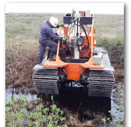
(left) MIP setup on a MarshMaster I. (above, below, and bottom left) Enviro Depot uses smaller Geoprobe units mounted on MarshMaster IIs.
