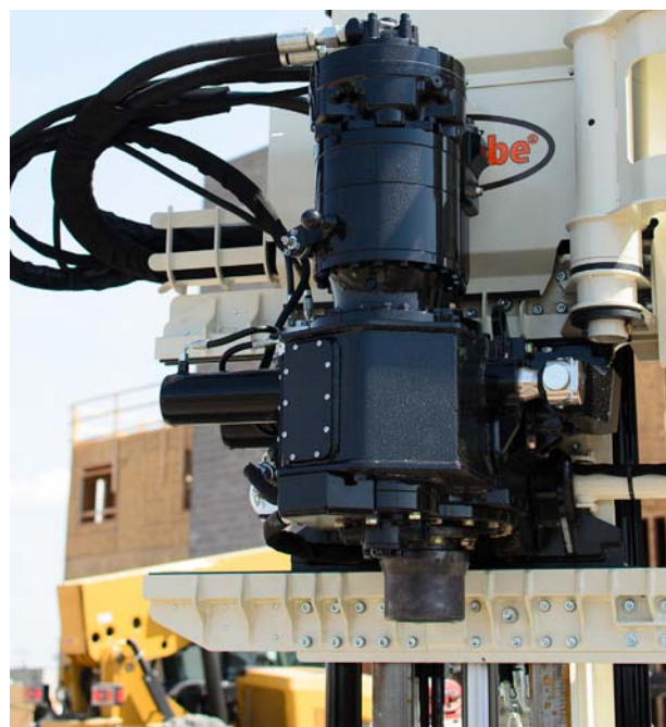
The centerline side-shift function of the 3230DT allows you to move the head to the side so you can work the inside diameter of the rod without moving the foot.
