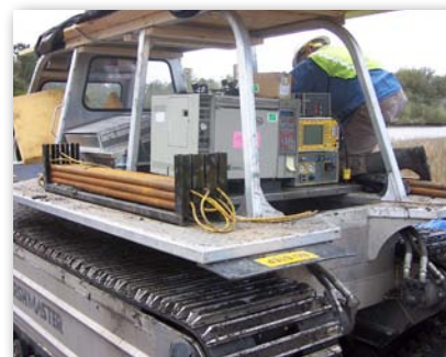
(left) MIP setup on a MarshMaster I. (above, below, and bottom left) Enviro Depot uses smaller Geoprobe units mounted on MarshMaster IIs.
