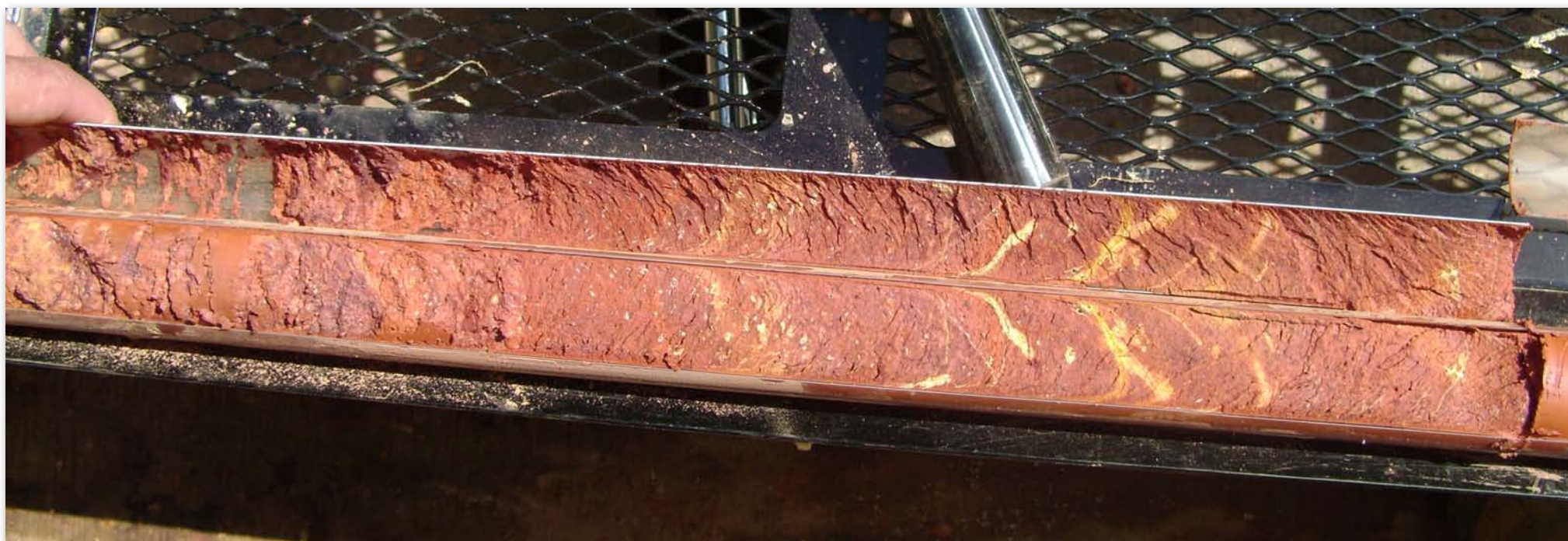
MC5 sample of Saprolite recovered at 98 ft. (30 m) bgs. Saprolite is a chemically-weathered rock which forms in the lower zones of soil profiles and represent deep weathering of the bedrock surface. The sample was collected by a field team in the jungles of Suriname using a Geoprobe® 8040DT with DT45 and MC5 tooling.
