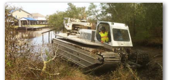
(left) MIP setup on a MarshMaster I. (above, below, and bottom left) Enviro Depot uses smaller Geoprobe units mounted on MarshMaster IIs.
