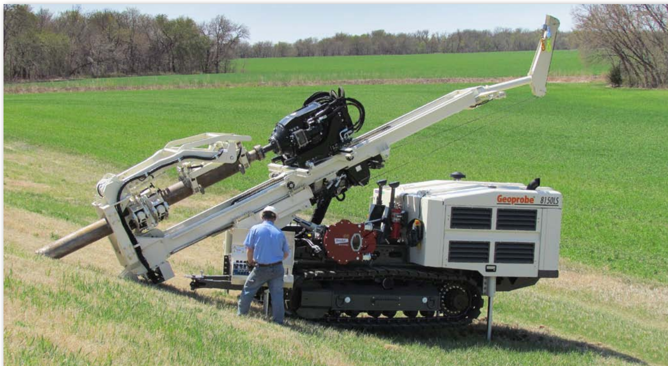
The 8150LS Sonic: a powerful, full-size sonic rig from Geoprobe®.
