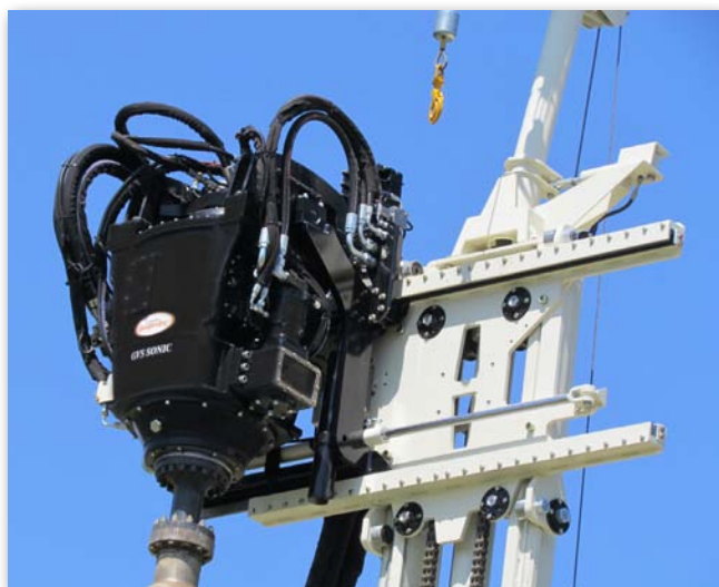
The NEW GV5 Sonic Head on the 8150LS is designed, built, and serviced by Team Geoprobe®. It has a theoretical dynamic force of 50,000 lb. at 150Hz, a substantial increase in power from our 8140 series sonics.
