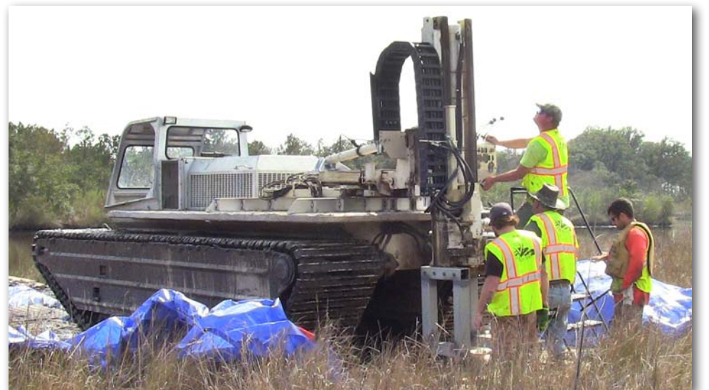
It floats and paddles! Enviro Depot took their 6600 machine mounted on a MarshMaster III (above and below) on its maiden voyage to complete 75 ft. MIP logs on a mud flat after traversing a small bayou. They subsequently collected groundwater samples from multiple intervals.
