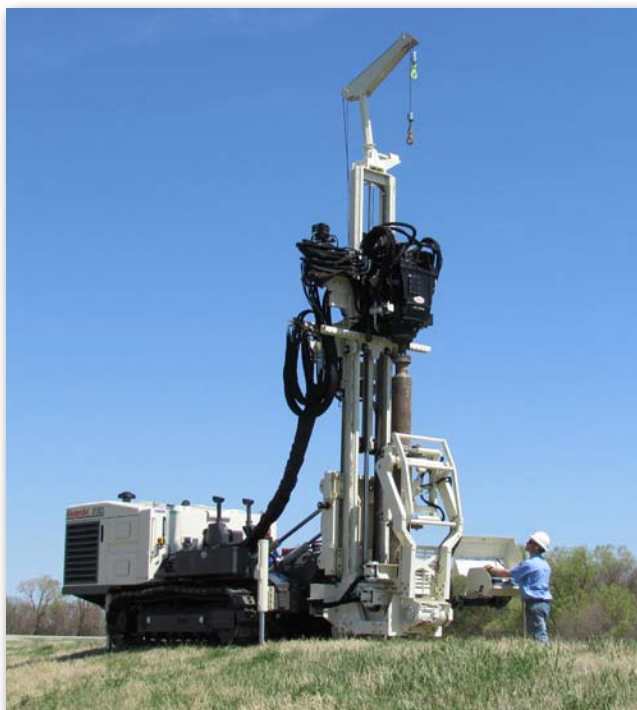
The new 8150LS features a 14-in. breakout option and a more powerful rod handler.
