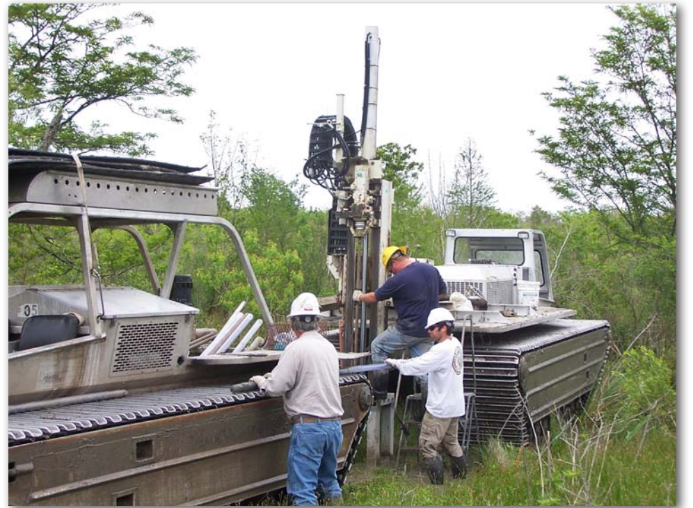
It floats and paddles! Enviro Depot took their 6600 machine mounted on a MarshMaster III (above and below) on its maiden voyage to complete 75 ft. MIP logs on a mud flat after traversing a small bayou. They subsequently collected groundwater samples from multiple intervals.
