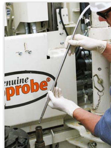
The SP22 Groundwater Sampler screen is deployed through the 2.25-in. probe rod string using Geoprobe® 1.25-in. Lightweight Center Rods (shown) or 0.75 in. PVC riser. Groundwater samples are collected from within the screen with a small-diameter bladder pump, mini bailer, or tubing and a check valve.
