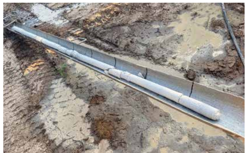
Top: Chris Foster, drill operations foreman, leverages power of DM250 to conduct wireline coring, increasing productivity on the kaolin mine. Bottom: Cores retrieved to find best clay quality to keep customers satisfied. The raw material will then be mined for dry kaolin clay used to make paper, ceramics, and medicines.
