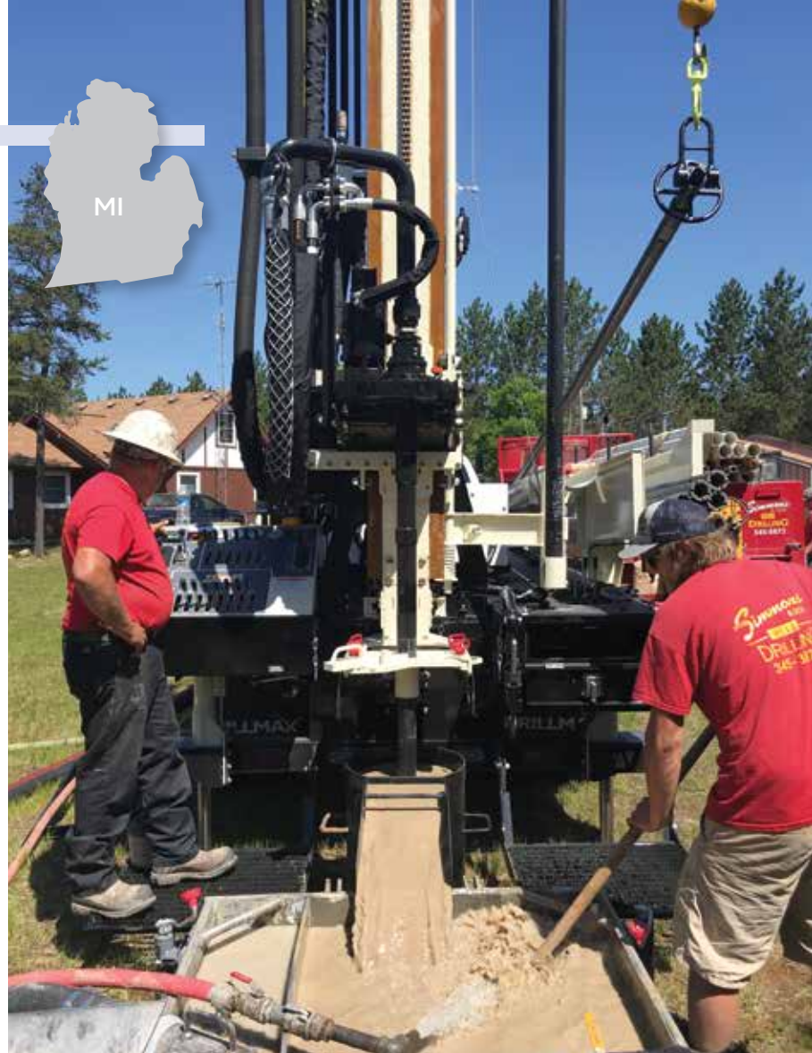
Small footprint and faster head speed combine for use on 90 percent of Simmons' jobs.
