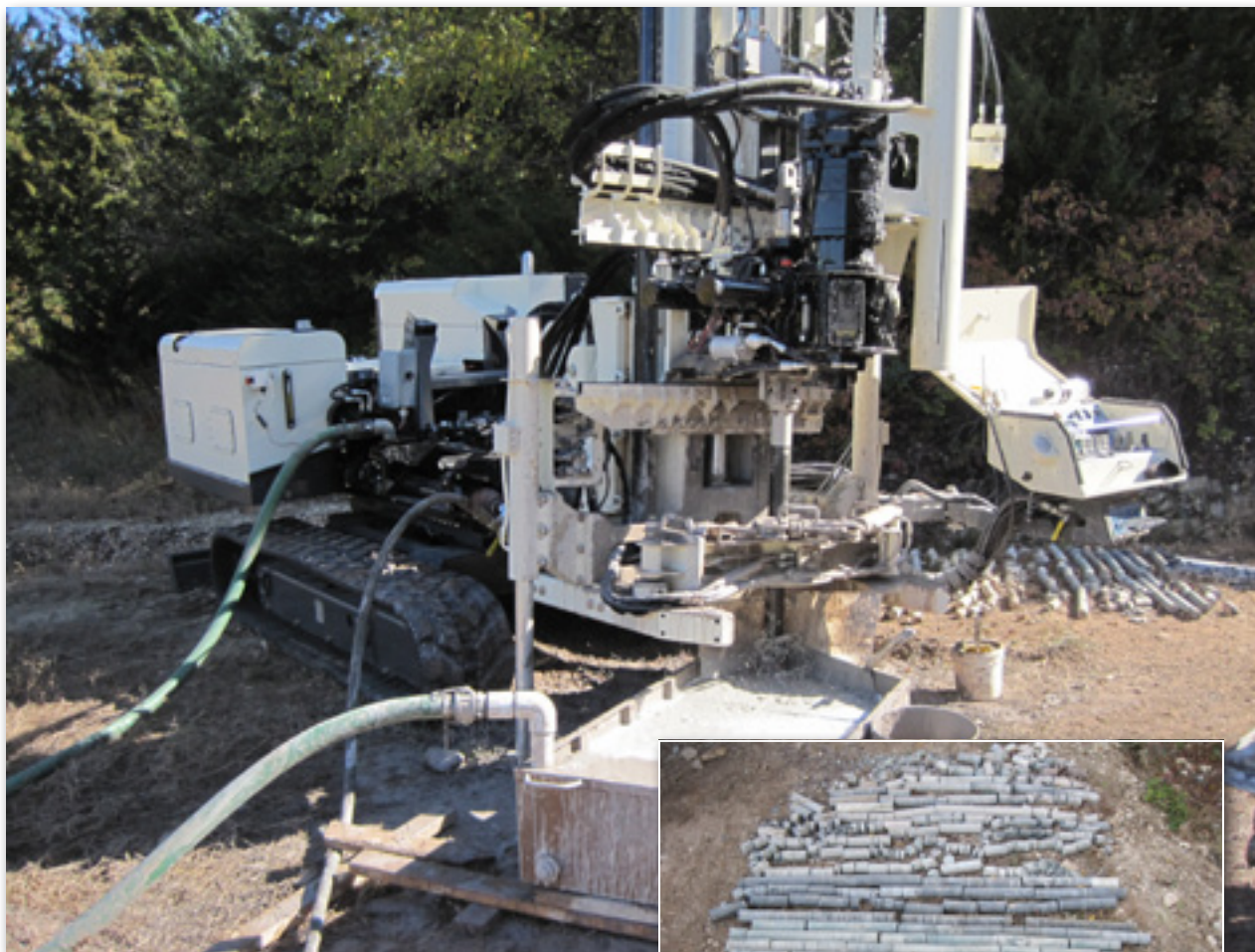
The 3230DT has what you need for diamond coring: outriggers stabilize the unit above the pan, multiple water pump and breakout options, head feed pressure control (weight-on-bit), and spindle rotation of up to 800 rpm.
