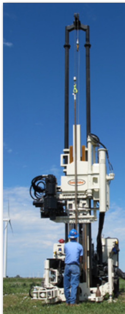
The CB6 Combo Head features a centerline sideshift function which allows you to move the head side-to-side so you can work the inside diameter of the rod without moving the machine.
