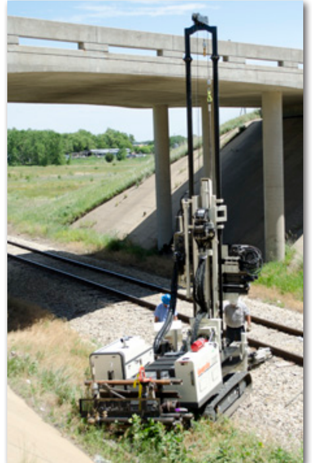
Oscillation +/- 10 degrees from center allows the field team to easily align the rig over the hole in tight and uneven conditions.
