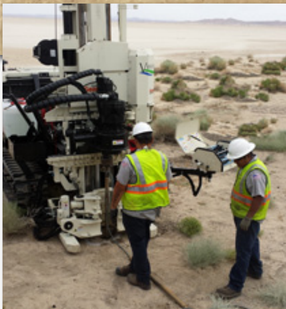
Alex Wesaw and Amner Ramos work with a Vironex 8040DT for MiHpt data collection (to 107 ft.) at a Department of Defense facility in southern California.
