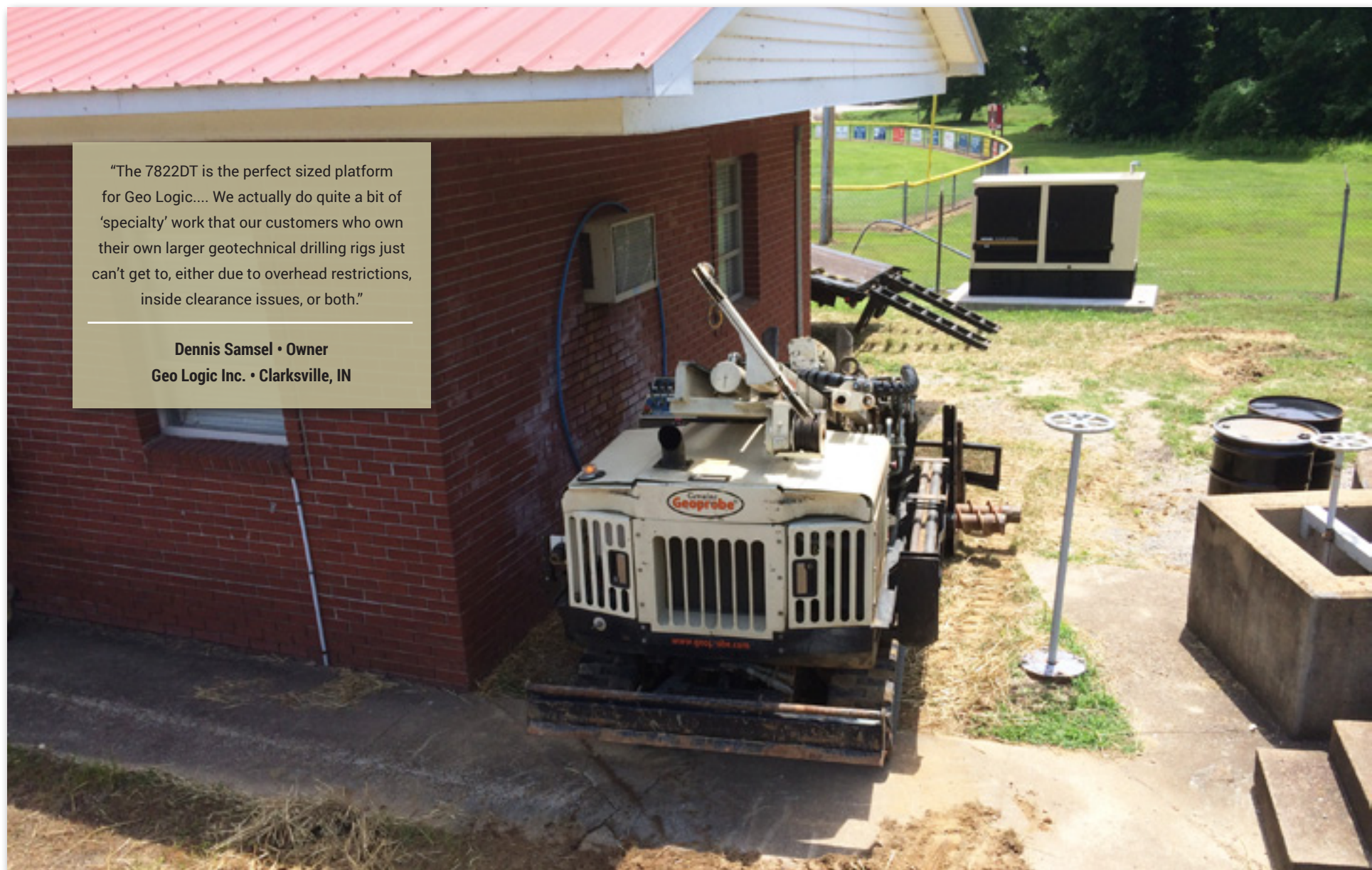
The 7822DT was a snug fit between the retention pond’s slope and the wastewater treatment plant’s building. There was no feasible way to get a truck-mounted rig, or any larger rig, to this location. The rig had to be oriented this way because the hoses would have hit the roof line if the rig had been turned around.
