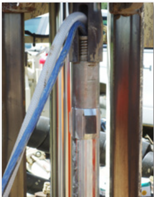
2.25 in. probe rods have a larger inner diameter allowing operators to run systems that require dual lines such as the pictured MiHpt with DI Grout Adapter. The blue line is a standard MiHpt trunkline; the white line is a separate grout line.
