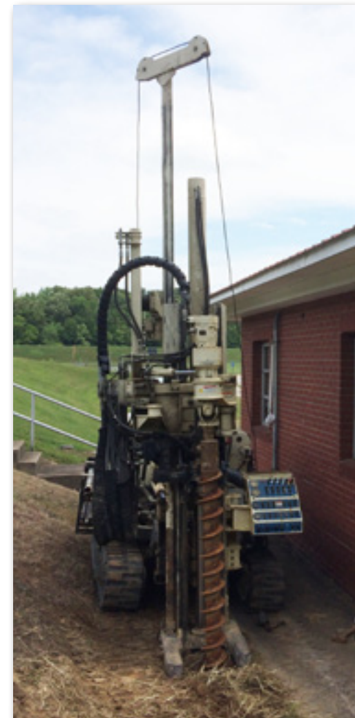
The 7822DT was a snug fit between the retention pond’s slope and the wastewater treatment plant’s building. There was no feasible way to get a truck-mounted rig, or any larger rig, to this location. The rig had to be oriented this way because the hoses would have hit the roof line if the rig had been turned around.
