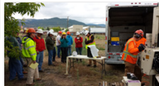
Ken Manchester (right) and Casey Briggs (behind) from Pioneer Technical Services in Butte, MT, advance an HPT probe into the subsurface at the former Caird Steel Works site in Helena, MT, as members of the MT DEQ observe the logging process. Three HPT logs were completed across the site, all showing high EC and high HPT pressure over most of the intervals logged, suggesting low permeability in the areas.
