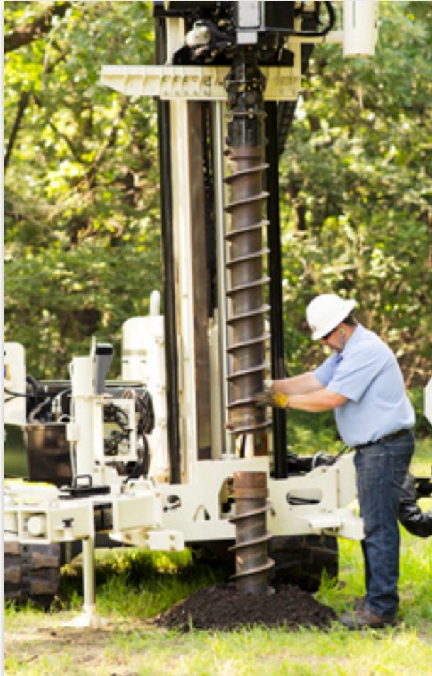
Drill mast outriggers provide a stable platform for rotary applications and the ability to hold and break inner rods above casing.
