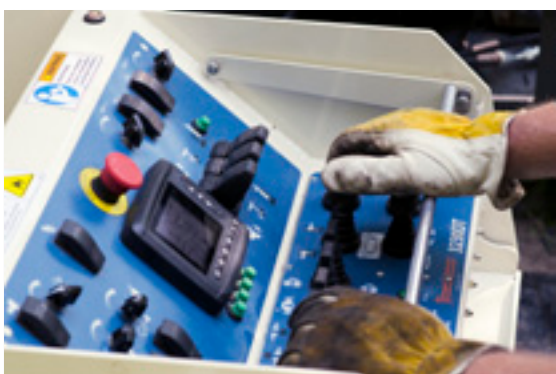
The moveable control panel makes it easy on the rig operator by providing a mixture of manual and electric-over-hydraulic controls. Electric controls allow for automation of several functions while the manual controls are used for basic positioning functions to reduce costs.
