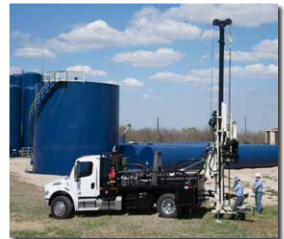
The truck-mounted 3200 makes mobilization to field sites easy and convenient.
