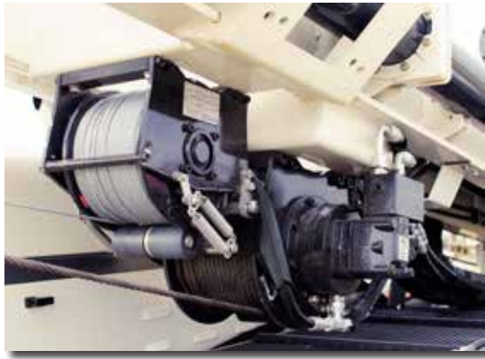
Dual winches mounted on 3230DT.
