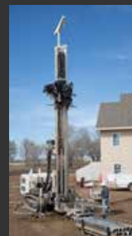
8250LS ... full-size rotary sonic, 20 ft Tooling 24 ft. 6 in. Head Travel
