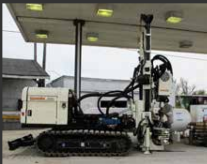
8140LC ... mid-size rotary sonic, Low Clearance Option 7 ft. 8 in. Head Travel
