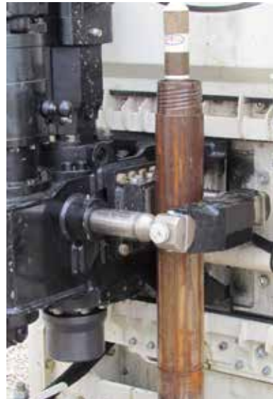
The built-in Head Clamp can handle the 80,000 lb. of the rig's pullback.
