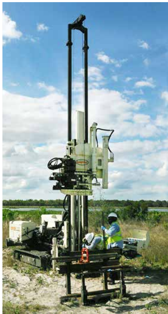
EnviroTek in Tampa, FL, uses a 3230DT to run high-speed wireline tooling at a Florida mining site.
