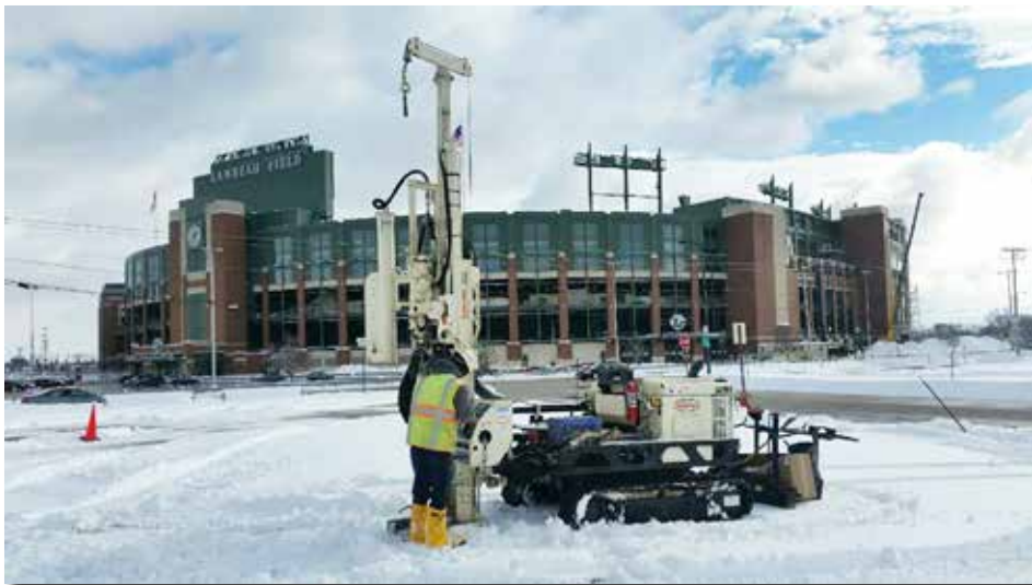
It's not every day you get to drill at the ball park. Tim Winkler, Project Manager for Gestra Engineering in Milwaukee, WI, uses their 7822DT to pull samples at Lambeau Field, home of the Packers. So, is the Pack back?
