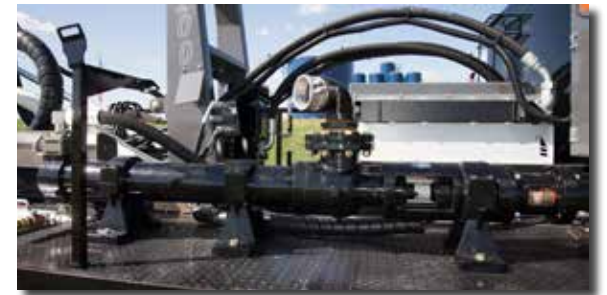
3200 equipped with a Moyno® 3L8 pump.
