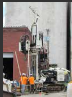
8140LS ... mid-size rotary sonic, Long Stroke Option 13 ft. 1 in. Head Travel
