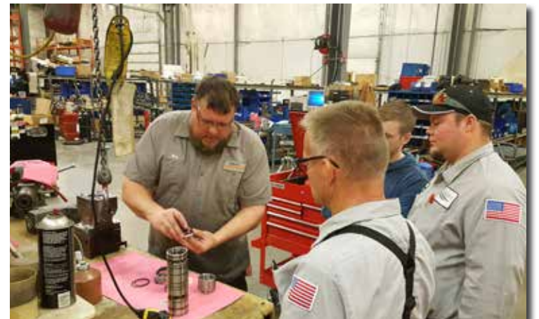
Mark Wessel, Geoprobe® Hammer Specialist, demonstrates to customers how to install a new seal kit to a GH60 Series percussion hammer.
