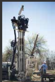
8150LS ... full-size rotary sonic, 10 ft. Tooling 13 ft. 1 in. Head Travel
