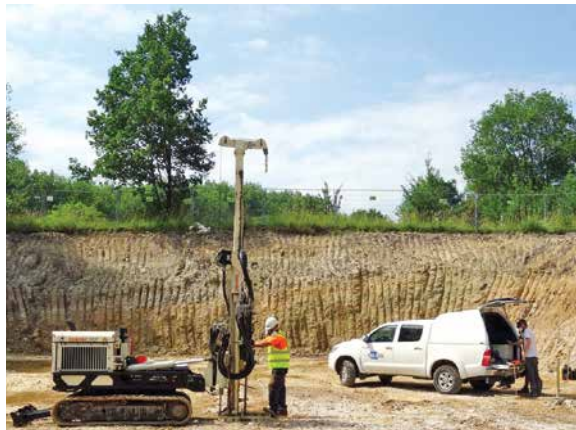
Above: OIP was used within the landfill body to characterize the layers of contamination. Left: An example of landfill profiling using OIP under visible light. Contaminated horizons are clearly visible (paint residues etc.)
