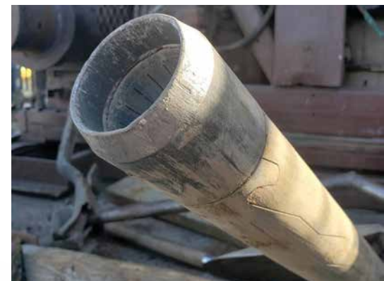
The shoes shown were just pulled from a job site after being driven to refusal on bedrock (30 to 50 blows with the 340-lb. auto drop hammer) in two, 35-foot borings. Blow counts were in the 20-40 range per 6 inches throughout the borehole, sampling every 2.5 to 10 feet, and then every 5 feet thereafter to refusal around 35 feet in total depth. The shoes look to be in fantastic shape even after multiple bedrock refusal drives.
