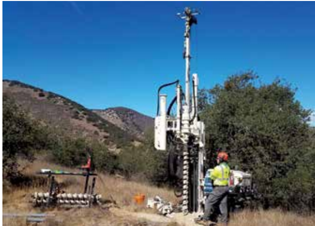
Exploration in reservoir fill abutment (left). Geoprobe® 7822DT installing 2-inch monitoring casing to 30 feet, in remote mountains (below).
