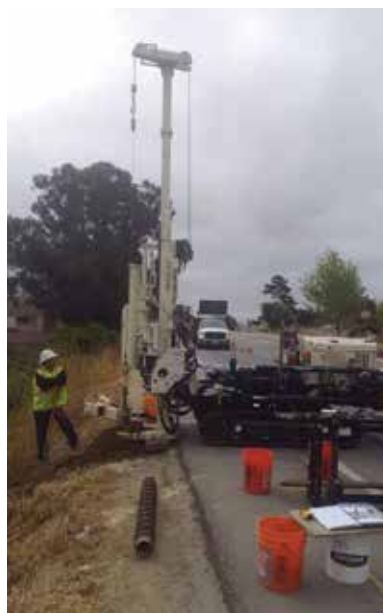
Geoprobe® 7822DT rotary wash drilling to 150 feet with 4.75-inch tri-cone (left). Exploration on top of fill edge with hollow stem, auto drop hammer, modified California samples and direct push Macro-Core® sampling to determine fill/native and native/sedimentary formation contacts (center). 7822DT hollow stem exploration for proposed sidewalks and road shoulder investigation on steep bank (right).
