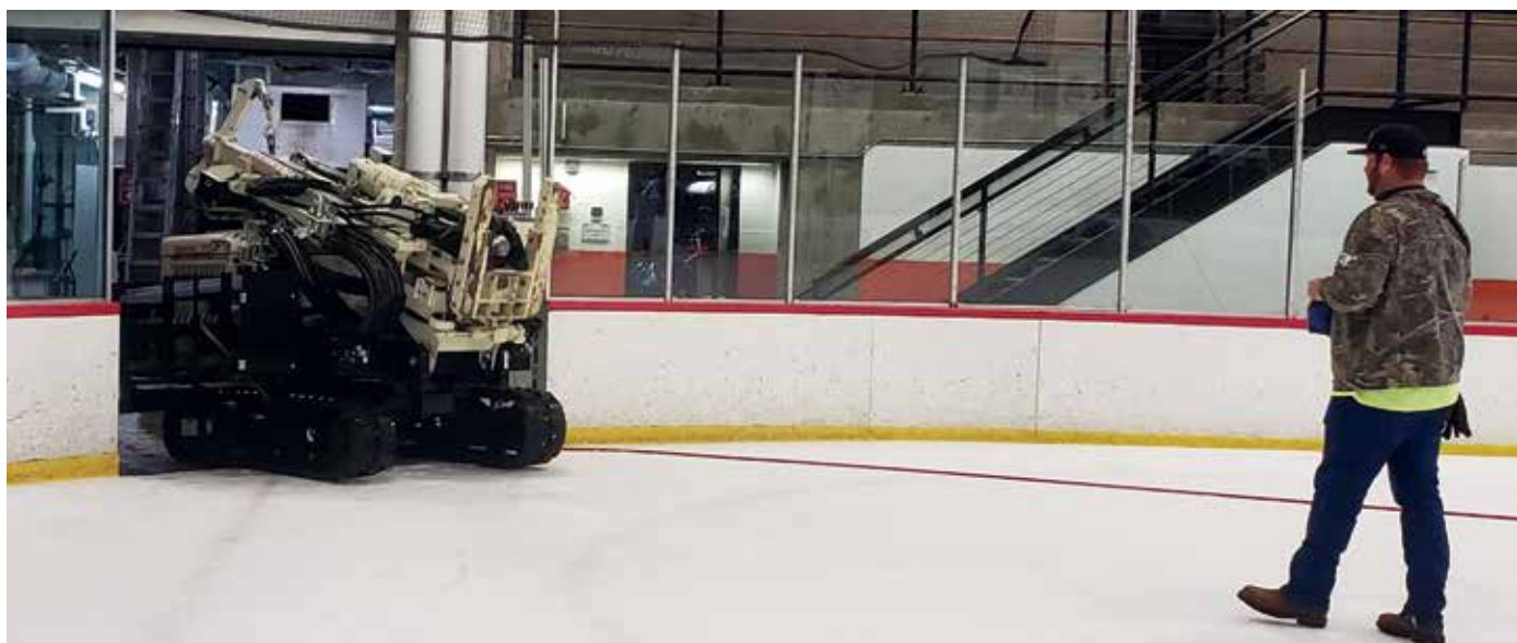
Gregg Drilling LLC conducts Macro-Core® sampling at the former Anaheim Ducks practice facility (left). They chose the Geoprobe® 7822DT for its narrow width, low track load on the ice surface (4.6 lb./in 2 ), rubber tracks, and ease of operation with the wireless remote. The fact that it was only three months old was also an advantage, keeping dirt from falling off the tracks onto the rink (right).
