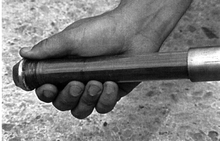
Figure 11. Removing the liner to recover the sample.
