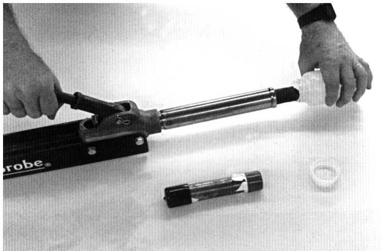
Figure 13. Extruding a sample in a metal liner using the AT659K manual extruder.
