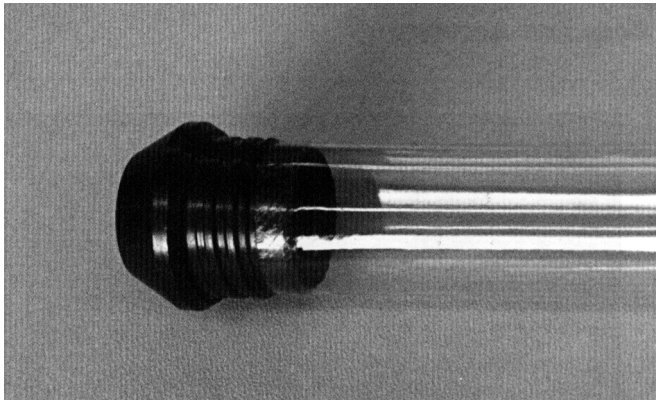
Figure 5. Liner fits snugly over interior end of cutting shoe.
