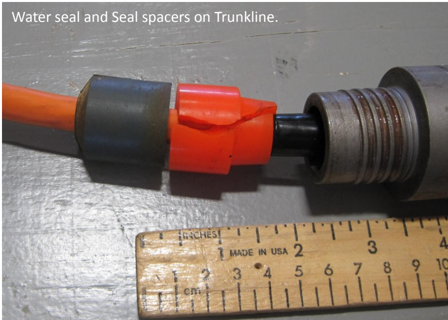
Trunkline pushed into connection tube, trunkline seal and spacers in place.
