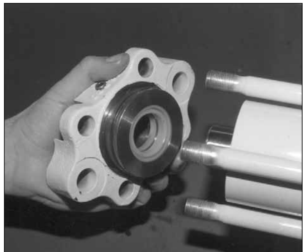
Fig. 6.10. Slide base plate onto side rods and piston.
