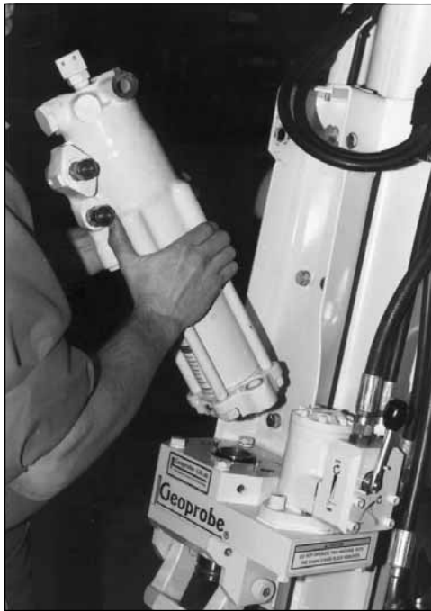
Fig. 8.1. Lower hammer member onto hammer alignment pins.
