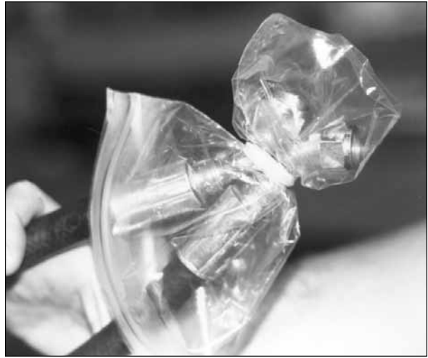
Fig. 8.6. Remove plastic bags or caps from hammer inlet return hoses.
