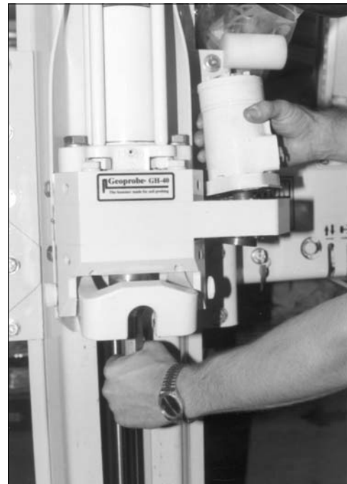
Fig. 14.4. Turn hex drive by hand or with 1" hex (a drill steel may be used) to achieve alignment.
