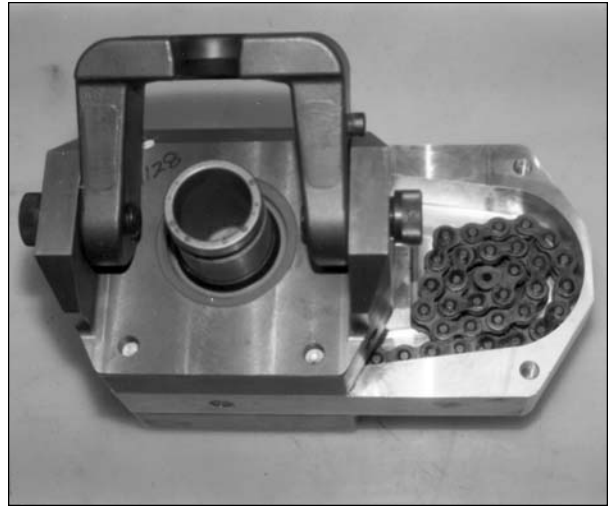
Fig. 16.4. Coil chain to fit into gear drive box.
