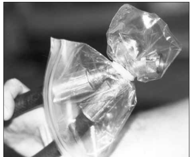
Fig. 4.4A. Cover ends on all hydraulic lines removed from hammer with small plastic bags. (Option 1)
