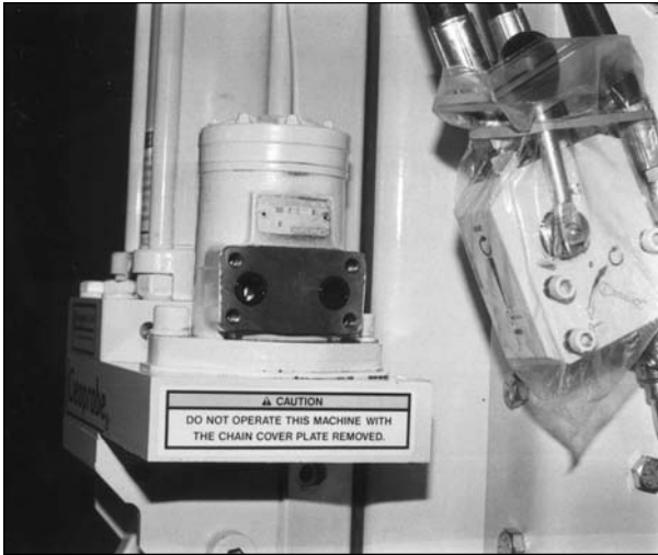
Fig. 13.10. Rotation valve should hang away from hammer.
