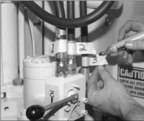
Fig. 11.3. Identify and tag hydraulic hoses going into valve body.
