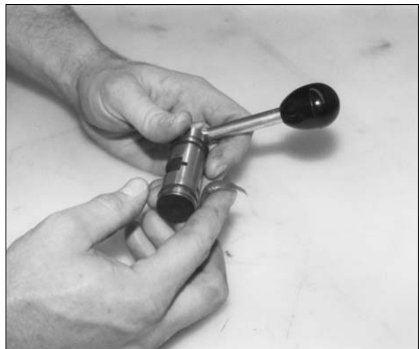
Fig. 12.5B. Apply hydraulic oil or grease to inside diameter of valve spool cylinder.
