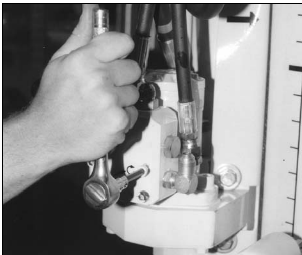
Fig. 12.9B. Attach hammer rotation valve to hydraulic motor.
