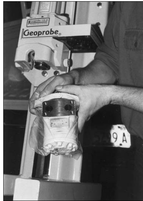
Fig. 13.14. Place entire hydraulic motor in a plastic bag.
