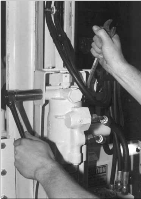
Fig. 8.5. Tighten top mounting bolt, lock washer, and nut.
