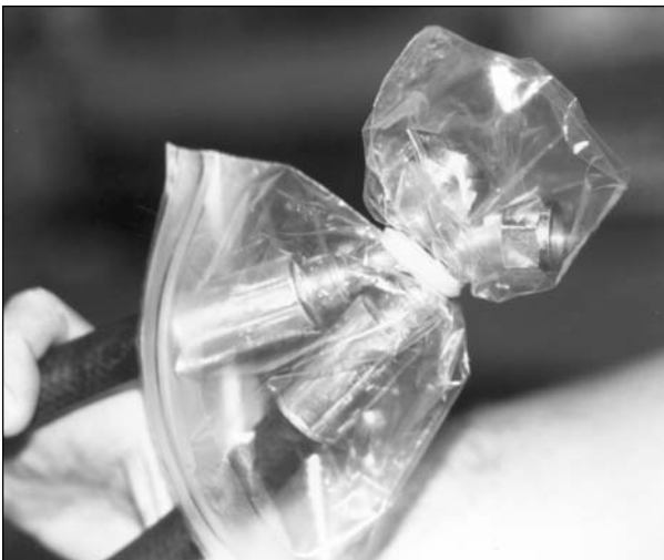
Fig. 11.5A. Cover hoses with small plastic bags. (Option 1)
