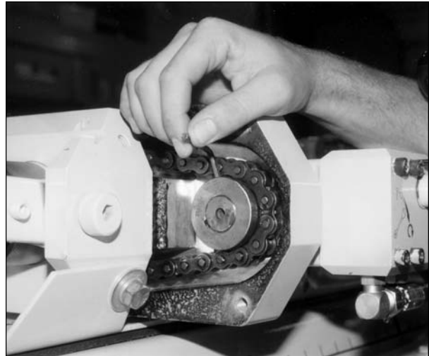
Fig. 15.4. Loosen 12-tooth sprocket set screws.
