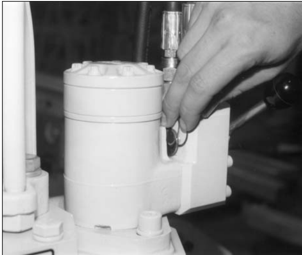
Fig. 10.14. Install retainer ring on spool between hydraulic motor and valve body.
