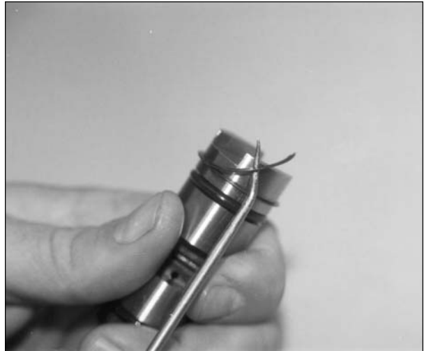
Fig. 11.13. Remove remaining retainer ring from valve spool.
