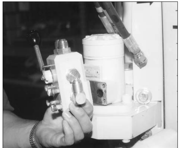
Fig. 12.9A. Hammer rotation valve is ready to be attached to hydraulic motor.
