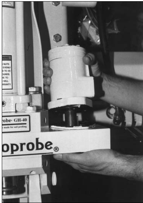
Fig. 13.13. Lift hydraulic motor off gear drive box.
