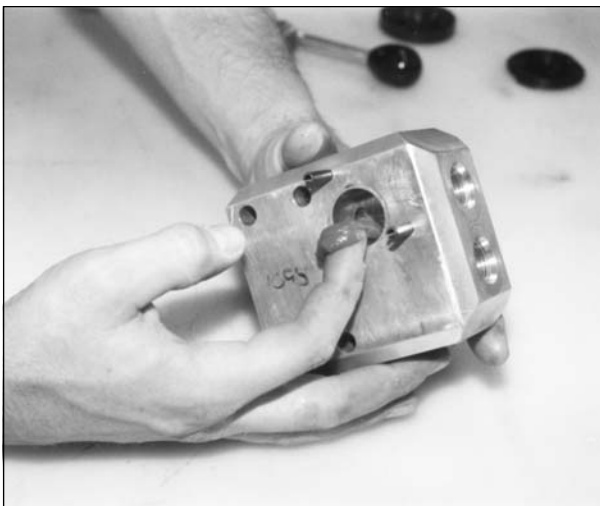
Fig. 12.5A. Apply hydraulic oil or grease to valve spool.
