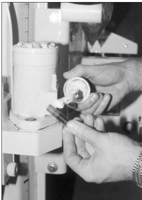
Fig. 14.7. Apply sealant to the socket head cap screws.
