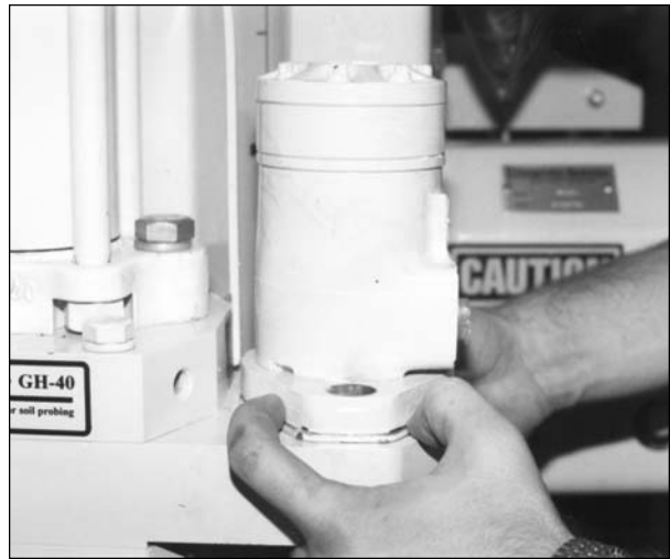
Fig. 14.6. Adjust hydraulic motor spacer for even fit.
