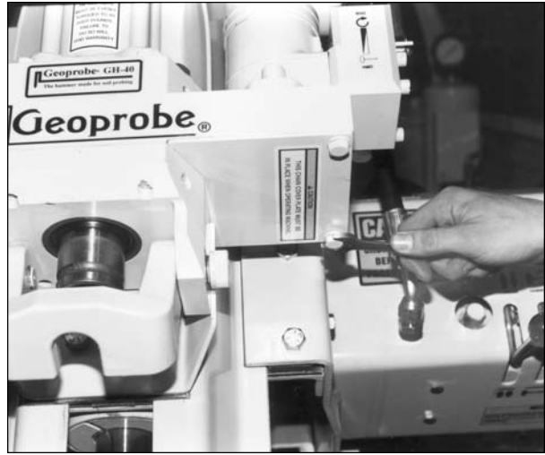
Fig. 15.2. Remove chain cover bolts and lock washers.
