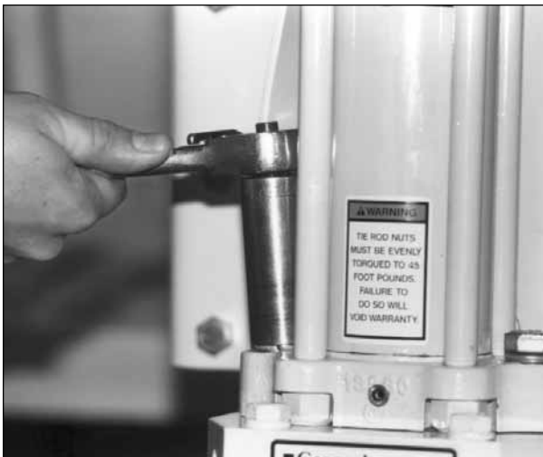
Fig. 4.6A. Loosen base plate bolt which secures hammer member to rotation member.
