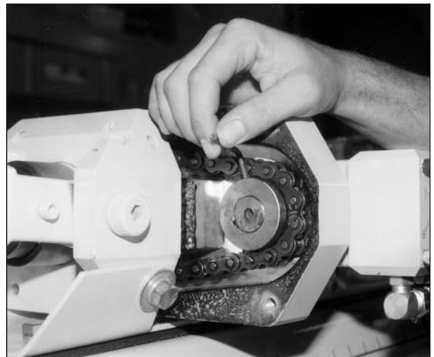
Fig. 14.12. Tighten 12-tooth sprocket set screws.
