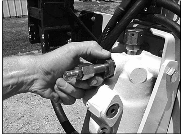
Fig. 7.6. Thread hex cap of charge valve adapter into nitrogen charge port until hand tight.
