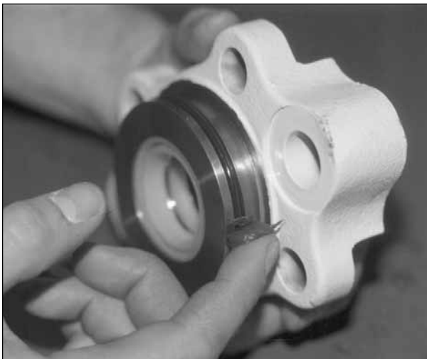
Fig. 6.7. Apply grease to installed base plate O-ring.
