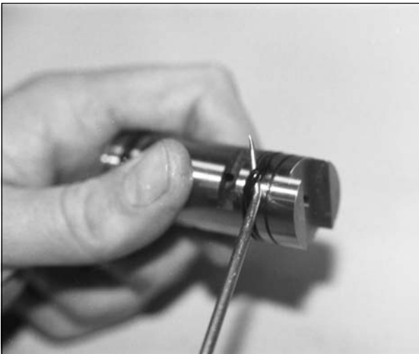
Fig. 11.14. Remove O-rings from valve spool.
