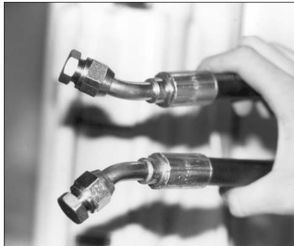
Fig. 11.5B. Plug hose ends with 8-MJ hydraulic fitting plugs. (Option 2)
