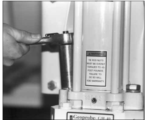
Fig. 8.4 Tighten base plate bolts evenly and securely.
