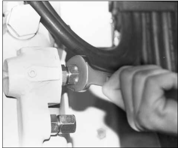
Fig. 4.5. Cap hammer inlet and return openings after hoses have been removed.
