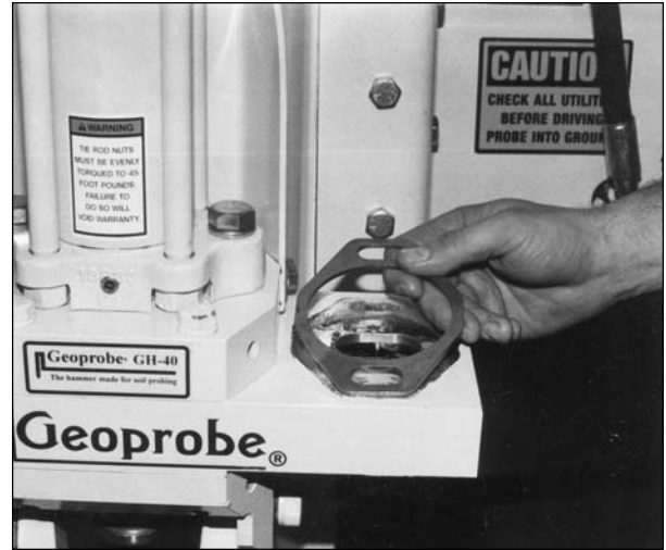
Fig. 14.2. Place hydraulic motor spacer on gear box and align bolt holes.
