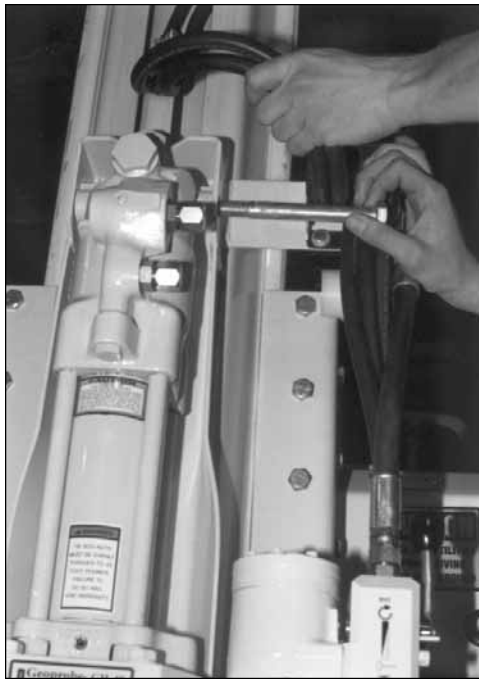
Fig. 8.3. Install top mounting bolt, lock washer, and nut.
