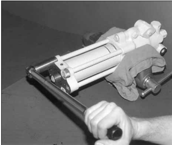
Fig. 6.13. First, torque side rod nuts to 30 foot pounds in a crisscross pattern; then torque to 45 foot pounds in a crisscross pattern.
