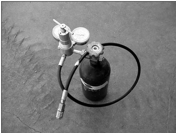
Fig. 7.1. Nitrogen gas cylinder with pressure regulator assembly.
