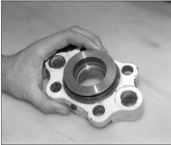
Fig. 6.1. Seal cavity on base plate should face upwards during installation.
