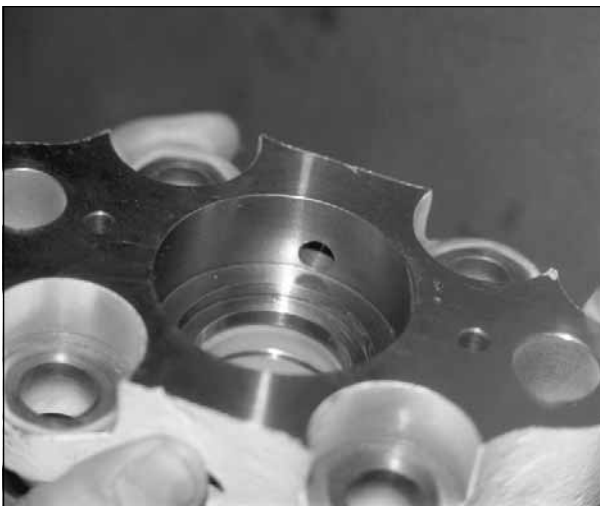
Fig. 6.9. Sub-seal vent port must face inlet and return fitting side of hammer.
