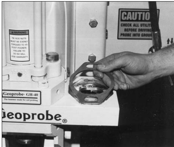
Fig. 13.15. Remove hydraulic motor spacer from gear drive box.
