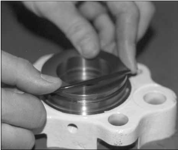
Fig. 6.5. Installation of base plate O-ring onto base plate.
