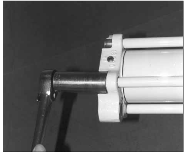
Fig. 6.12. Side rod nuts must be installed loosely and evenly.
