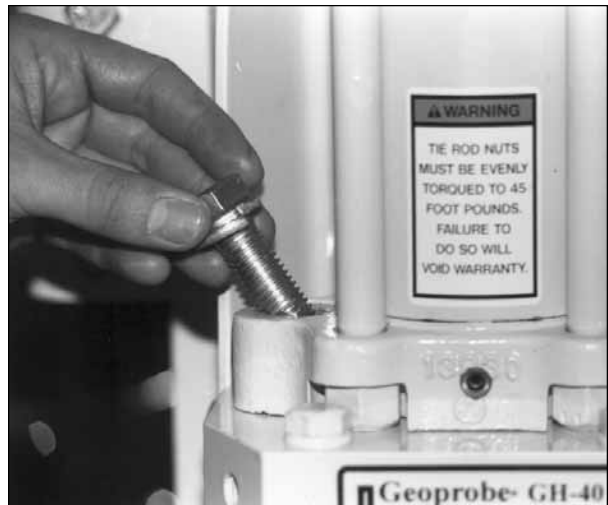
Fig. 4.6B. Remove hammer base plate bolts.
