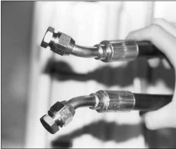
Fig. 4.4B. Plug ends on all hydraulic lines with 8-MJ plugs. (Option 2)
