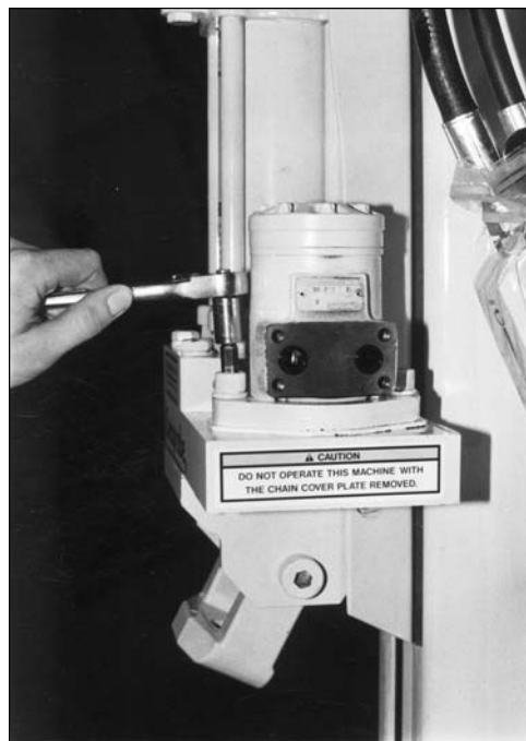
Fig. 14.8. Securely tighten socket head cap screws.
