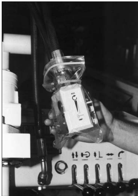
Fig. 13.7. Place hammer rotation valve in plastic bag and securely close.
