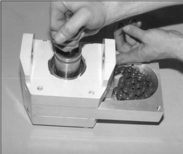
Fig. 16.5. Feed end of drive chain into and around hex drive gear using a drill steel.
