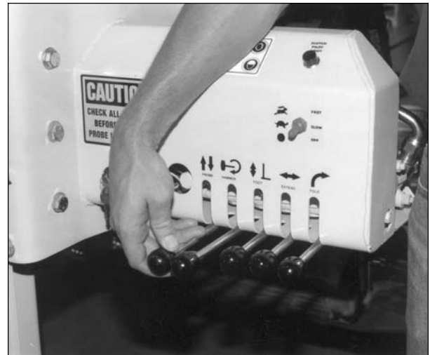
Fig. 11.2. Move hydraulic levers on control panel to relieve pressure in lines.
