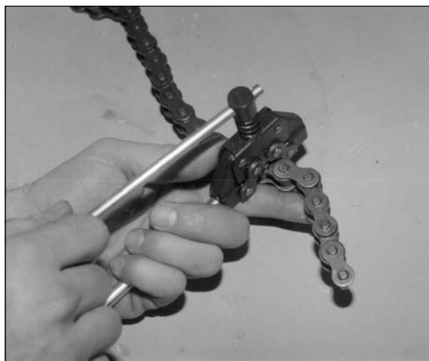
Fig. 16.1. Cut new section of #50 drive chain with chain detacher.
