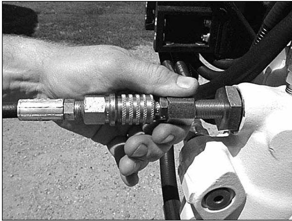
Fig. 7.11. Unthread the charge valve adapter center stem out from the hex cap.
