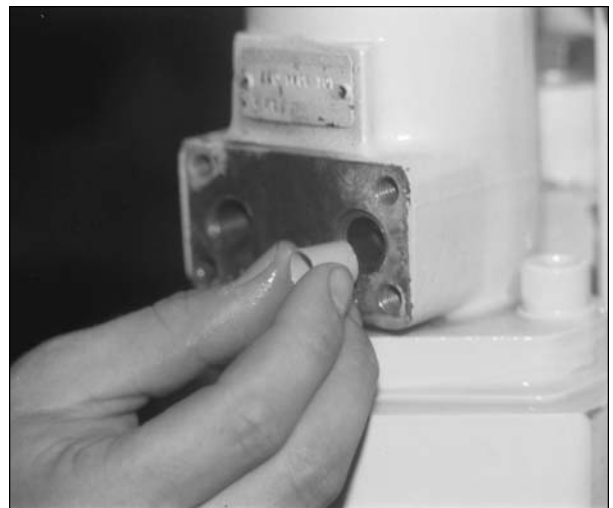
Fig. 13.9. Plug hydraulic motor oil ports with plastic plugs.
