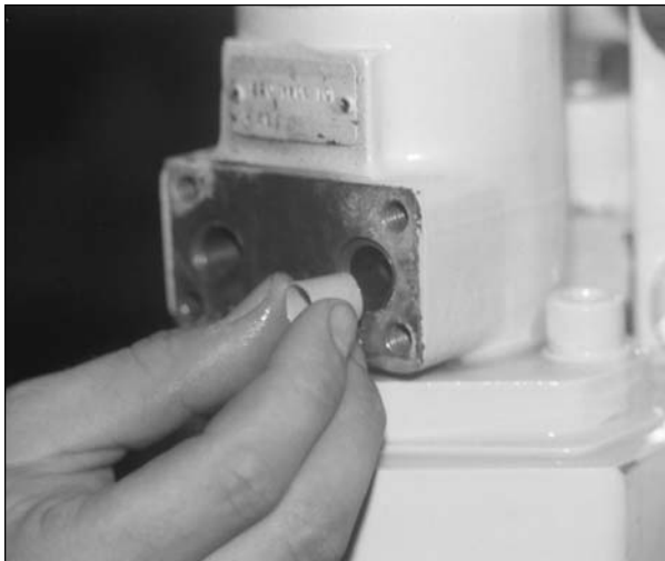
Fig. 11.9A. Plug hydraulic motor oil ports with plastic plugs. (Option 1)
