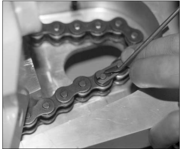
Fig. 15.12. Remove connector link keeper.
