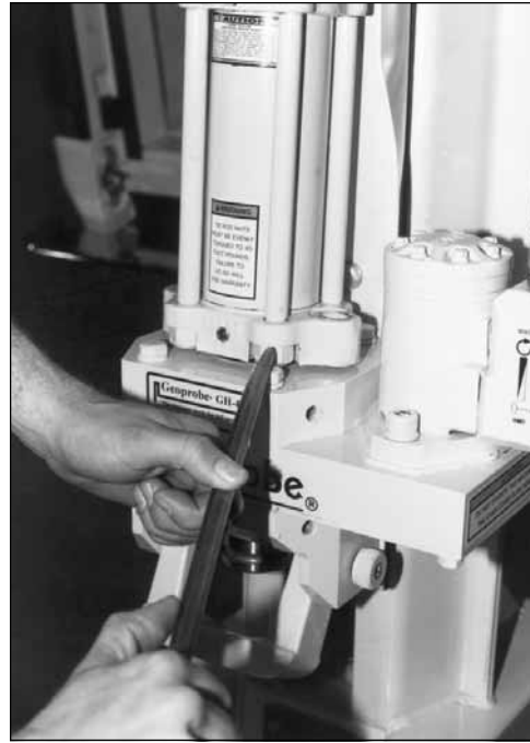
Fig. 4.8. Loosen hammer member from lower (rotation) member.
