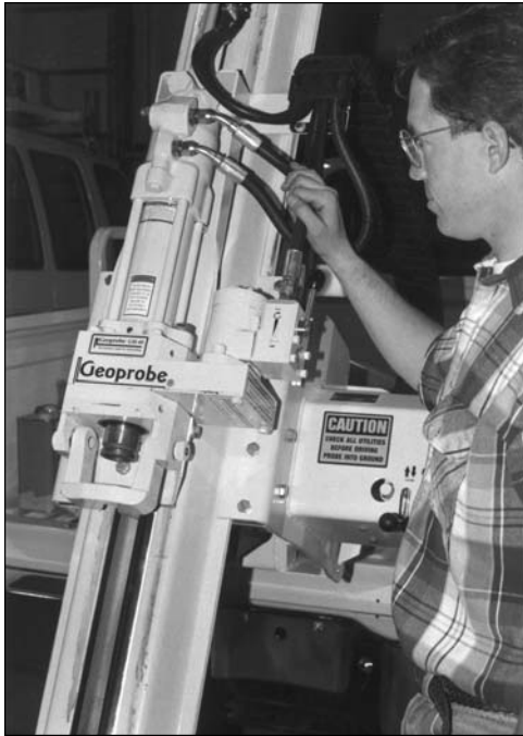
Fig. 13.1. Position GH-40 Hammer to chest height for hydraulic motor removal.
