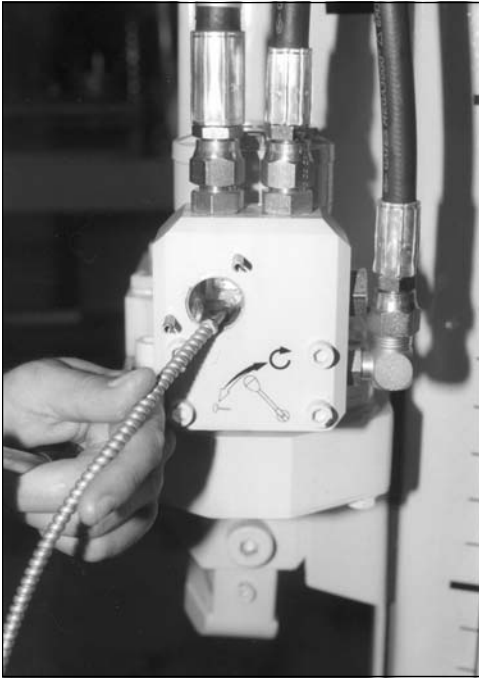
Fig. 10.8. Lubricate valve spool cylinder.
