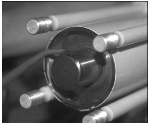
Fig. 6.8. Lubricate exposed surface of hammer piston.
