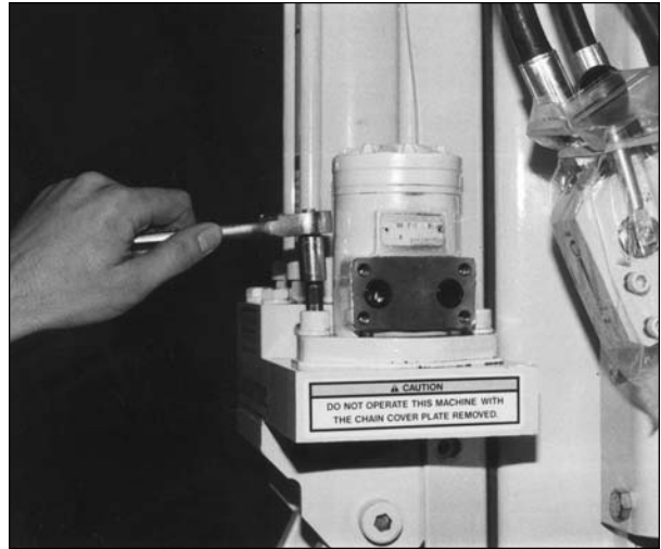
Fig. 13.11A. Loosen socket head cap screws from hydraulic motor mounting holes.
