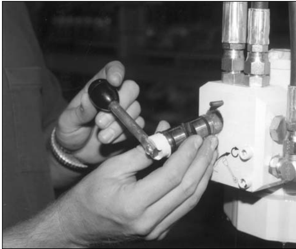
Fig. 10.6. Remove spool from valve body.
