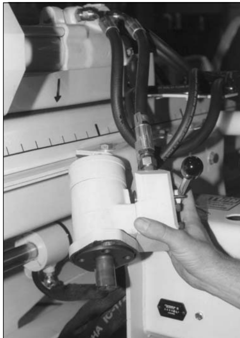
Fig. 15.9. Rest hydraulic motor against control panel.
