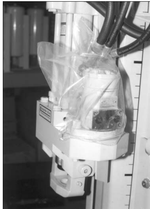
Fig. 11.9B. Enclose hydraulic motor in a plastic bag. (Option 2)
