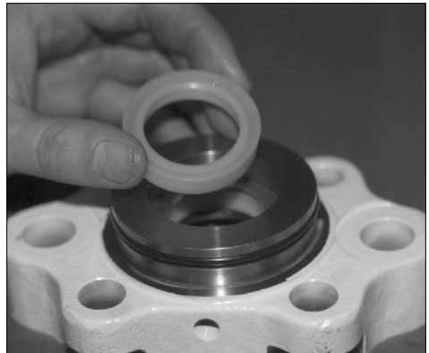
Fig. 6.4. Push cup seal onto seal washer.
