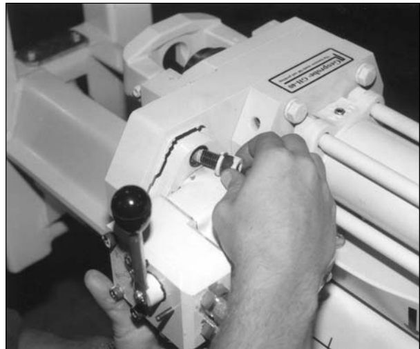
Fig. 15.6. Remove socket head cap screws.
