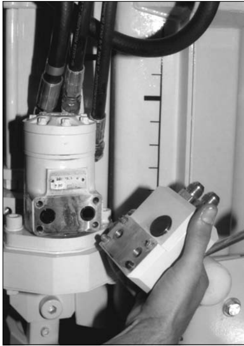
Fig. 11.7. Pull valve away from hydraulic motor.
