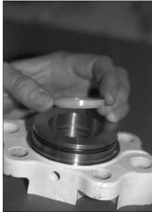
Fig. 6.2. Push "D" or "H" wiper into bottom seal cavity.
