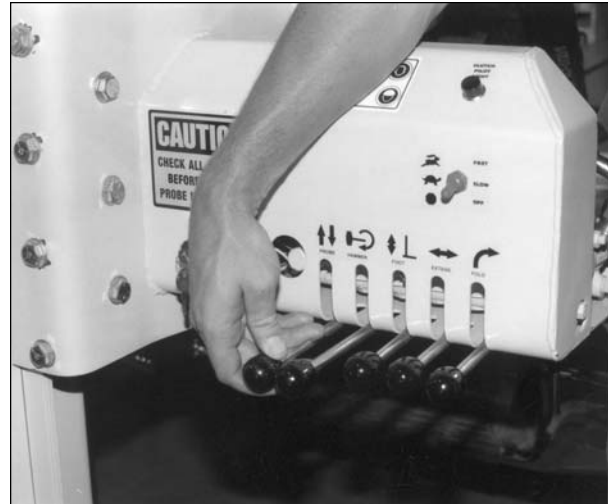
Fig. 10.2. Move hydraulic levers on control panel to relieve pressure in lines.
