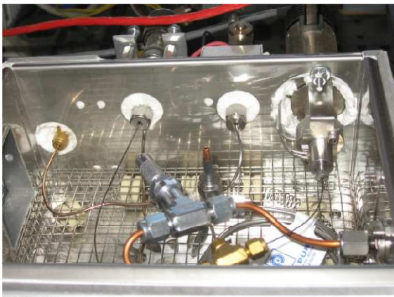
Figure 6: GC Oven plumbing of detectors: XSD, FID & PID
