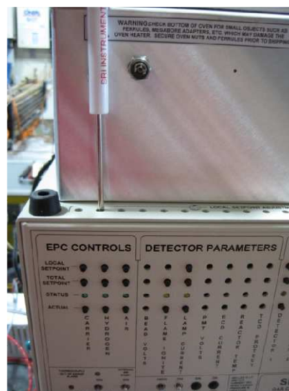
Figure 4 Adjusting the H 2 flow for the FID
