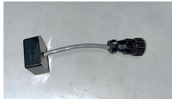
Figure 2: The Test Load (MN203898) is used to check the pneumatic slug test instrumentation.
