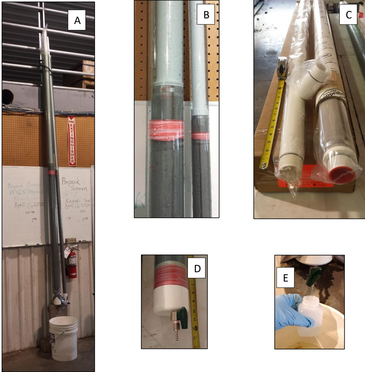
Photograph 1: Prepack screen PFAS rinsate test set up. A) Bench set up of both the 3" clear PVC and 1.5" clear PVC standpipes with prepack well assemblies in place, filled with PFAS free water. Duct tape used to hold standpipes on blocks to facilitate sampling from valve. B) Close up showing the slim 2" prepack screen with riser and the 0.75" prepack with riser in respective standpipes filled with PFAS free water. (C) Components of the 1.5" prepack well assembly used for extraction test. Taken from retail stock as packaged for delivery to clients. (D) Close up of stainless steel valve used for sampling from standpipe. (E) Filling sample bottle with water for PFAS analysis. Note: A liberal amount of Teflon® tape (pink in photos) was required on the PVC fittings of the standpipe casing to prevent leaks under positive head pressure.
