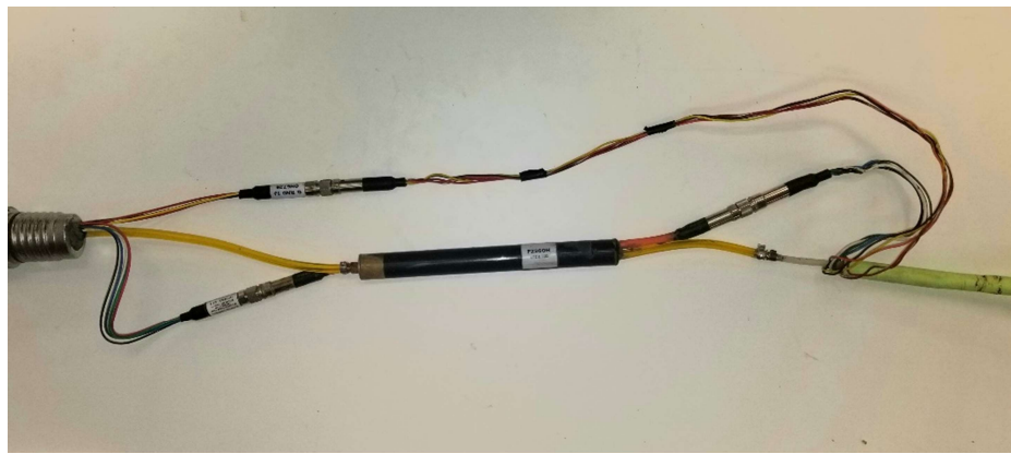
Figure 4.4 OIP Probe, OIP Power Supply and OIP Trunkline Connections
