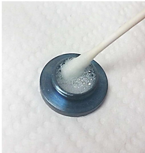
Figure 6.3 Cleaning the OIP Window is soapy water
