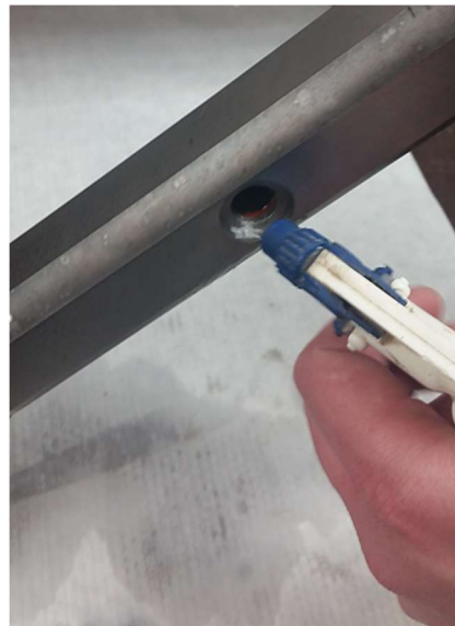
Figure 6.2: Flushing the optical cavity with alcohol
