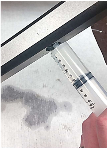
Figure 6.1: Flushing the optical cavity with water
