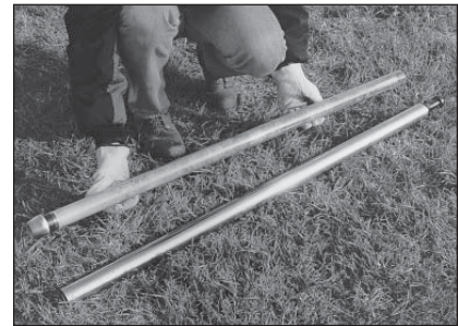
Figure 4.34. Macro-Core® liner filled with soil core.
