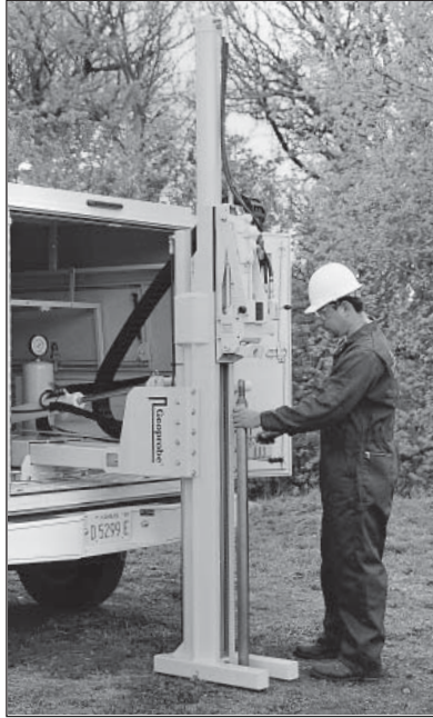
Figure 4.24 MC Sampler positioned for driving into subsurface.
