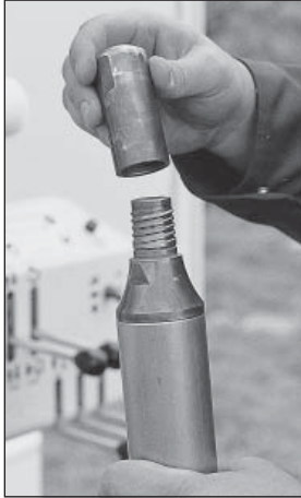
Figure 4.23. Thread drive cap onto sampler drive head.
