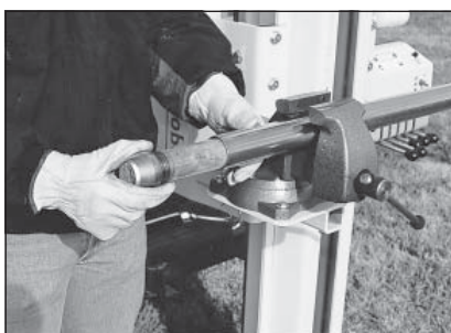
Figure 4.39. Removing filled liner with sample tube held in machine vise.
