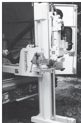
Figure 4.40. Machine vise mounted directly on Geoprobe Soil Probing Unit.
