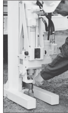
Figure 4.26. Hook hammer latch onto pull cap.
