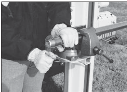
Figure 4.38. Removing MC Cutting Shoe with sample tube held in machine vise.
