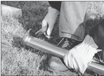
Figure 4.32. Loosening the MC Cutting Shoe with the MC Combination
