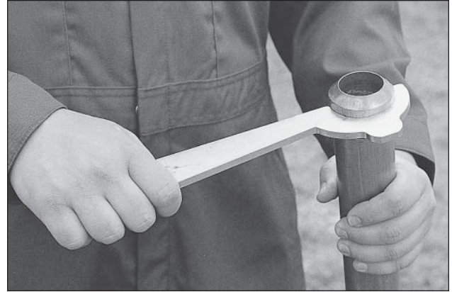
Figure 4.6. Tighten MC Cutting Shoe with MC Combination Wrench.
