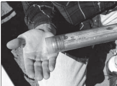
Figure 4.35. MC Piston Rod Point Assembly is retrieved from top of liner.
