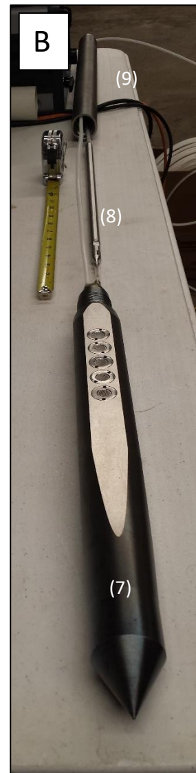
Photograph 1: Bench setup of the GWP 1.75 system for PFAS rinsate testing. Components include: Photo A: (1) HPT Flow Module, includes pump, flow meter, valves, internal plumbing, pressure meter, pressure gauge, water inlet line, bypass valve, bypass line, etc. (2) 60 ft HDPE water supply line with HPT pressure sensor behind flow module (3) MB6120 12V pump actuator (4) Assembled GWP 1.75 probe and syringe pump inside 2" PVC standpipe (5) 120 ft of ¼" HDPE sample line (6) Carboy of PFAS free water provided by Alpha Labs. Photo B: (7) GWP 1.75 Probe with 20 screened injection ports (8) syringe pump (9) connection tube with water supply line and sample line routed through it.
