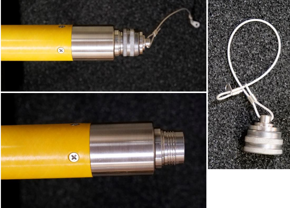
Figure 5: Dart probe with cap in place (top) and with cap removed (bottom). Cap is shown on right.
