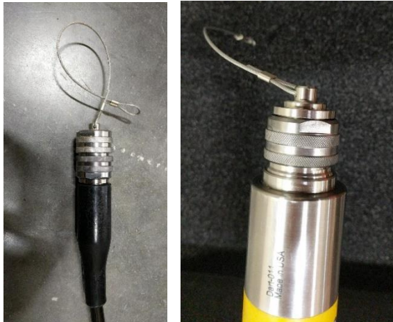
Figure 18: Protective caps in place on cable head (left) and probe (right).
