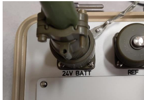
Figure 14: Connection from External Battery Cable to Control Unit "24V BATT" Port.
