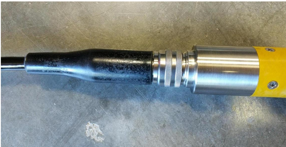
Figure 9: Logging cable attached to Dart probe.
