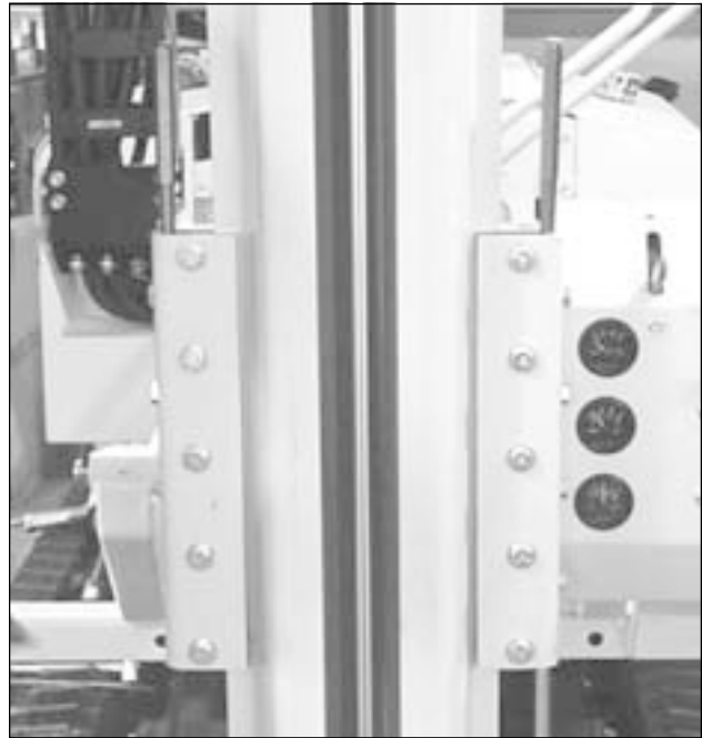
Figure 5: Adjust the center slides so that the foot is centered on the fold bracket and aligned with the vertical axis of the machine.
