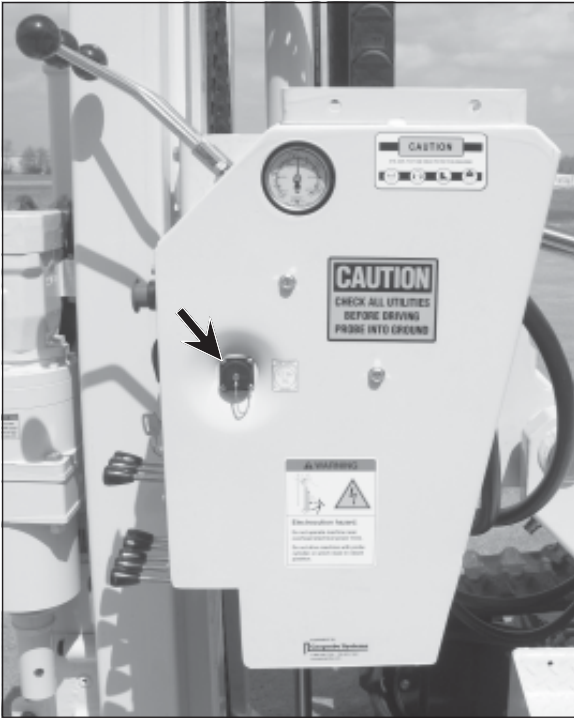
Figure 1: Geoprobe® direct push machines are equipped with 12VDC outlet receptacles (arrow).
